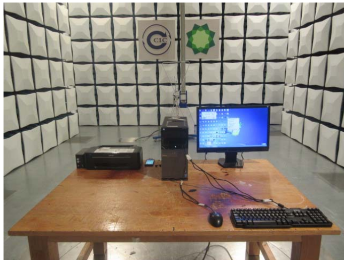
Radiated Emission (above 1GHz) Connect to PC
