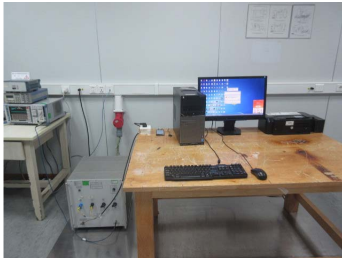
Radiated Emission (30MHz-1GHz) Connect to PC
