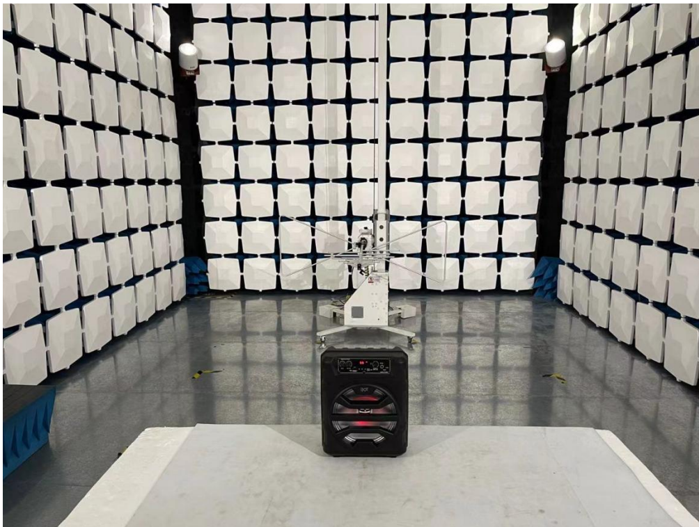
Below 1GHz for radiated emission test setup
