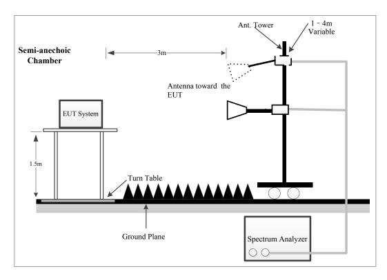
The radiated emissions were performed in the 3 meters distance, using the setup accordance with the ANSI C63.10-2020. The specification used was the FCC 15.209, and FCC 15.247 limits.
