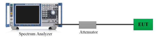
A short RF cable with low cable loss connected to the EUT antenna port, which was provided by manufacturer. The insert loss of this RF cable/attenuator was offset into the setting of test equipment.
