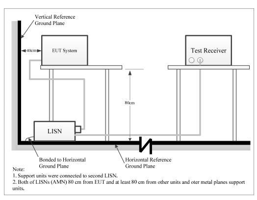
The setup of EUT is according with per ANSI C63.10-2020 measurement procedure. The specification used was with the FCC Part 15.207 limits.
