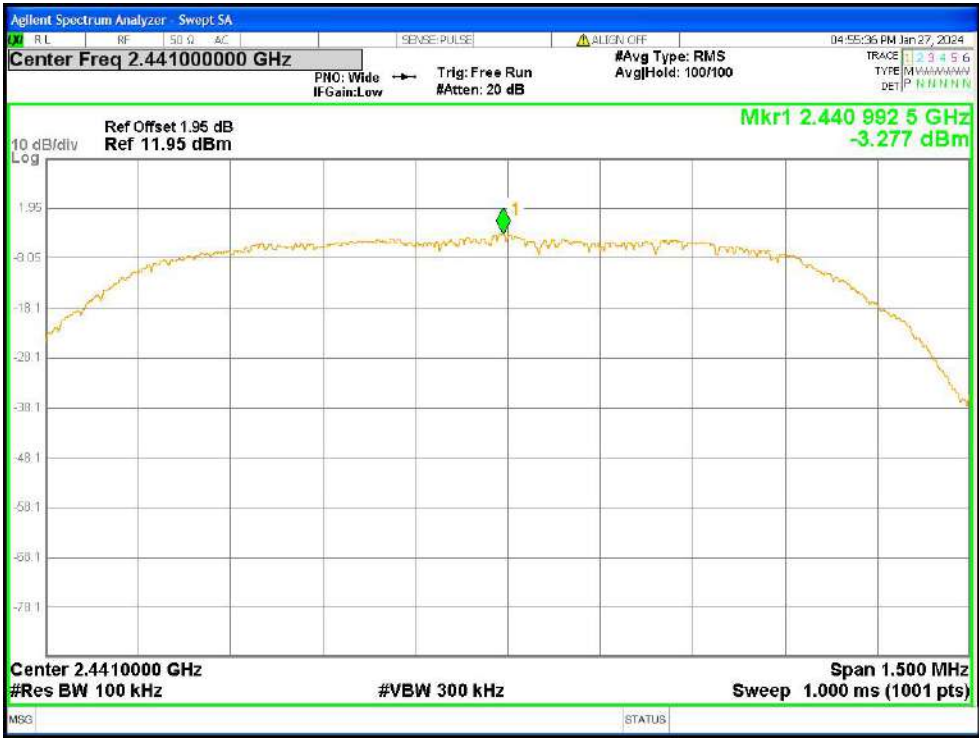
Tx. Spurious NVNT 2-DH5 2441MHz Ant1 Ref
