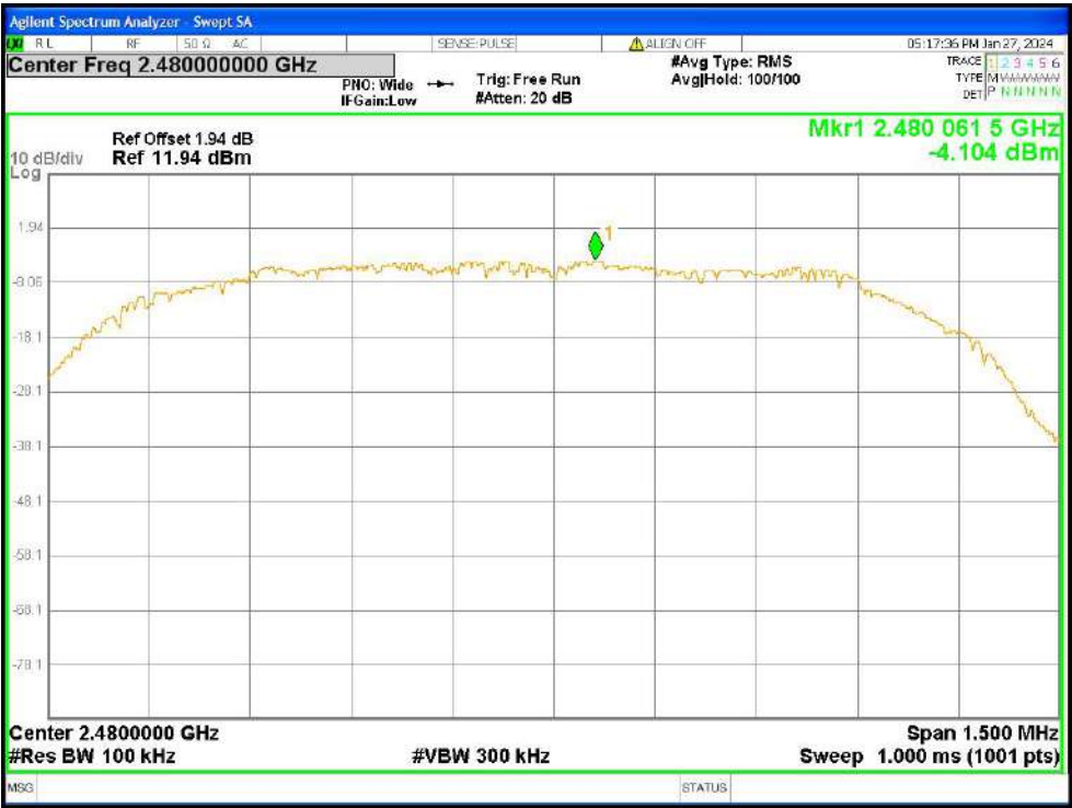
Tx. Spurious NVNT 3-DH5 2480MHz Ant1 Ref
