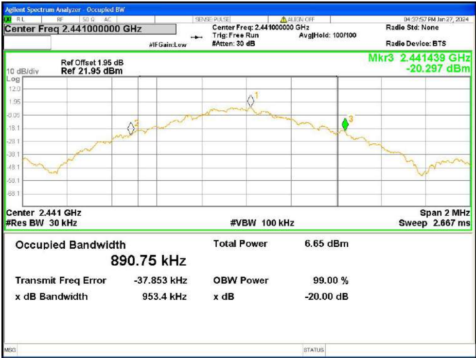
-20dB Bandwidth NVNT 1-DH5 2441MHz Ant1
