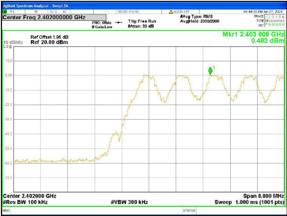
Band Edge(Hopping) NVNT 1-DH5 2402MHz Ant1 Hopping Ref
