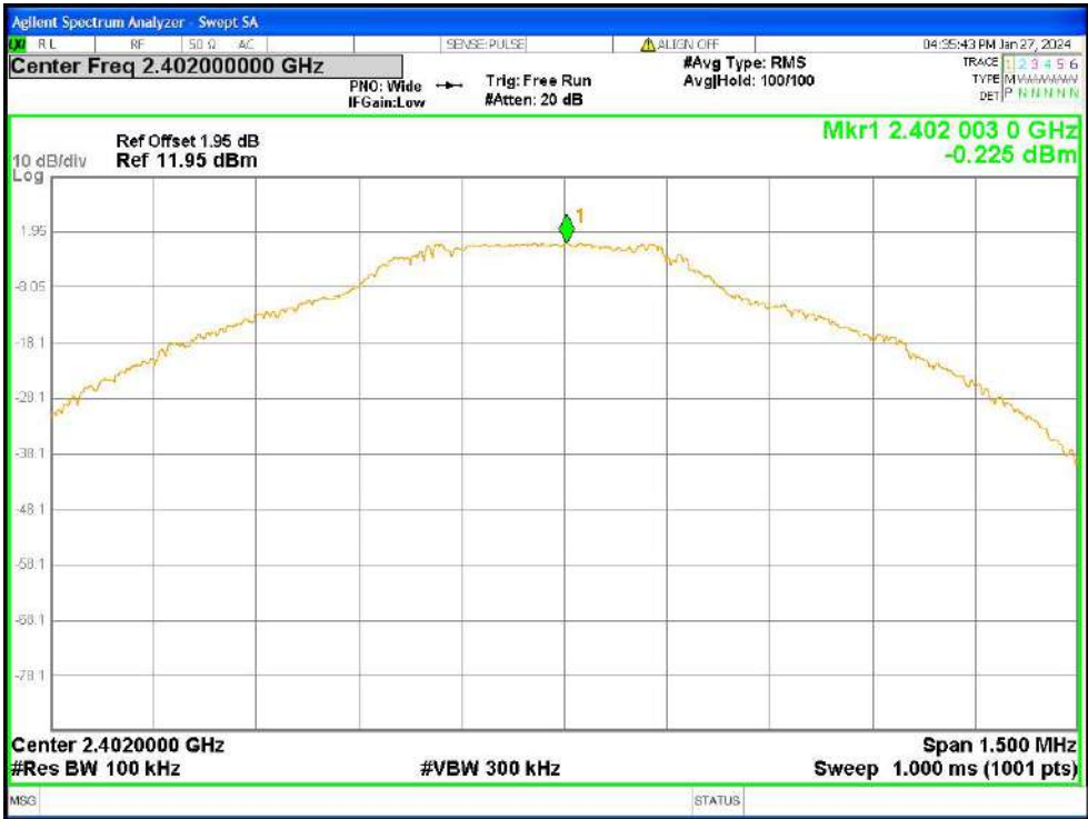
Tx. Spurious NVNT 1-DH5 2402MHz Ant1 Ref
