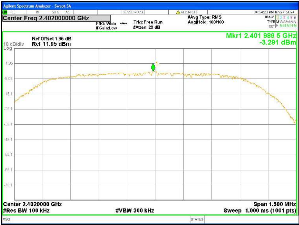
Tx. Spurious NVNT 2-DH5 2402MHz Ant1 Ref
