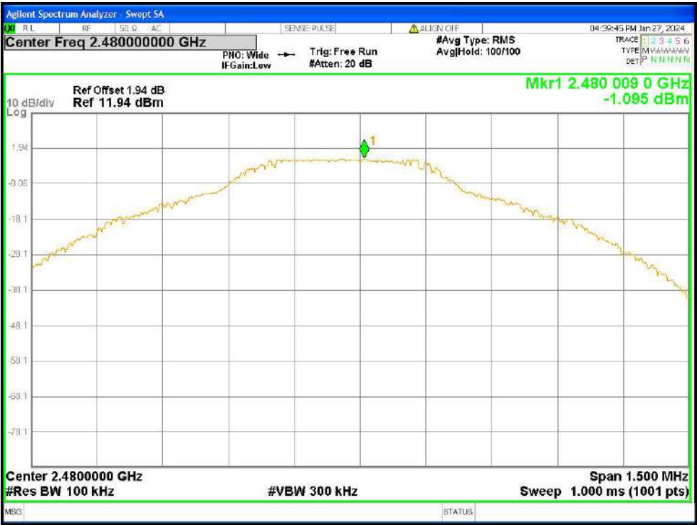
Tx. Spurious NVNT 1-DH5 2480MHz Ant1 Ref
