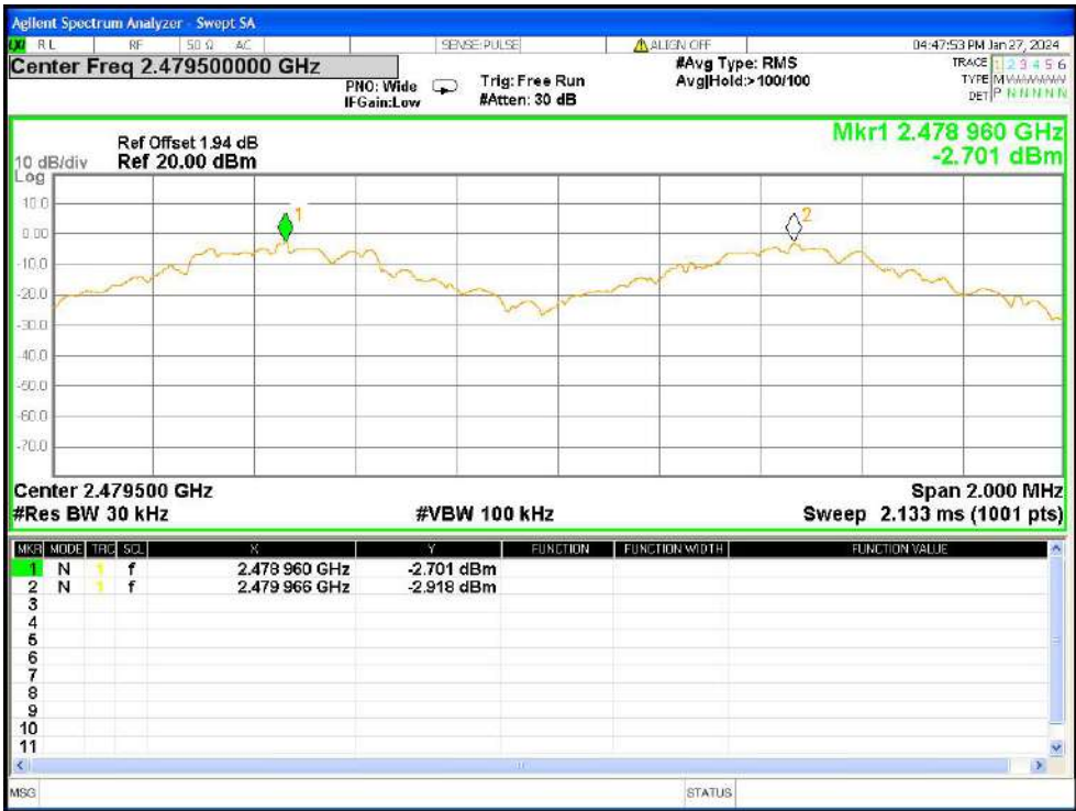
CFS NVNT 1-DH5 2480MHz Ant1
