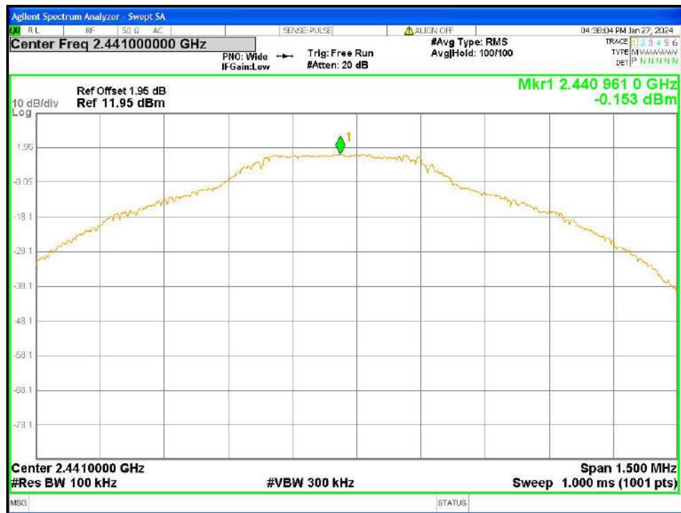
Tx. Spurious NVNT 1-DH5 2441MHz Ant1 Ref
