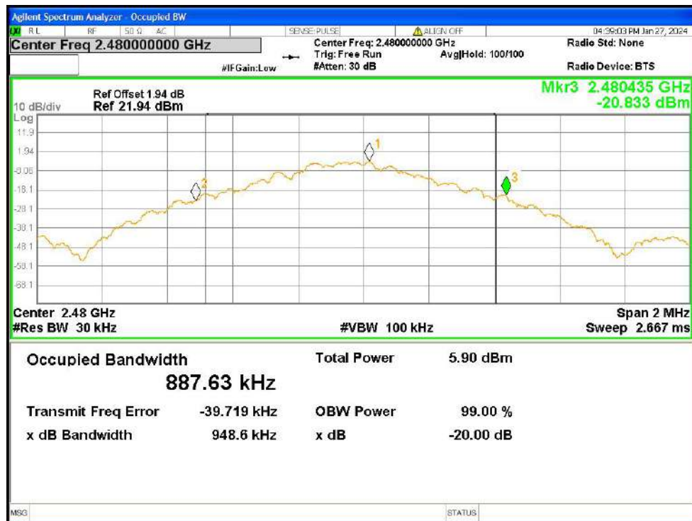
-20dB Bandwidth NVNT 1-DH5 2480MHz Ant1
