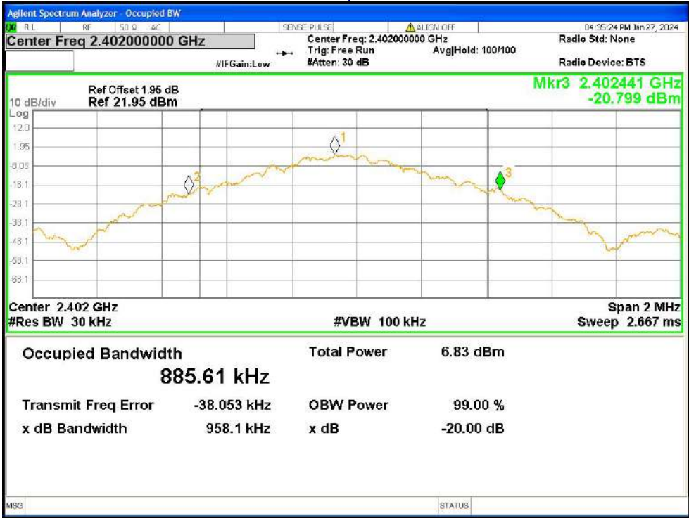
-20dB Bandwidth NVNT 1-DH5 2402MHz Ant1
