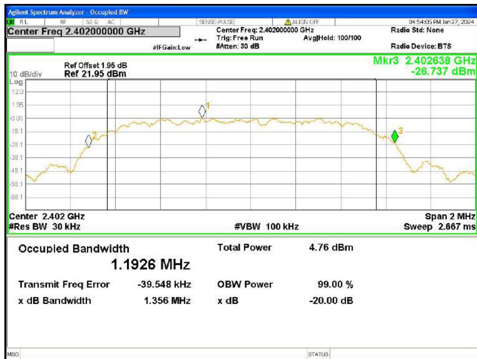
-20dB Bandwidth NVNT 2-DH5 2402MHz Ant1
