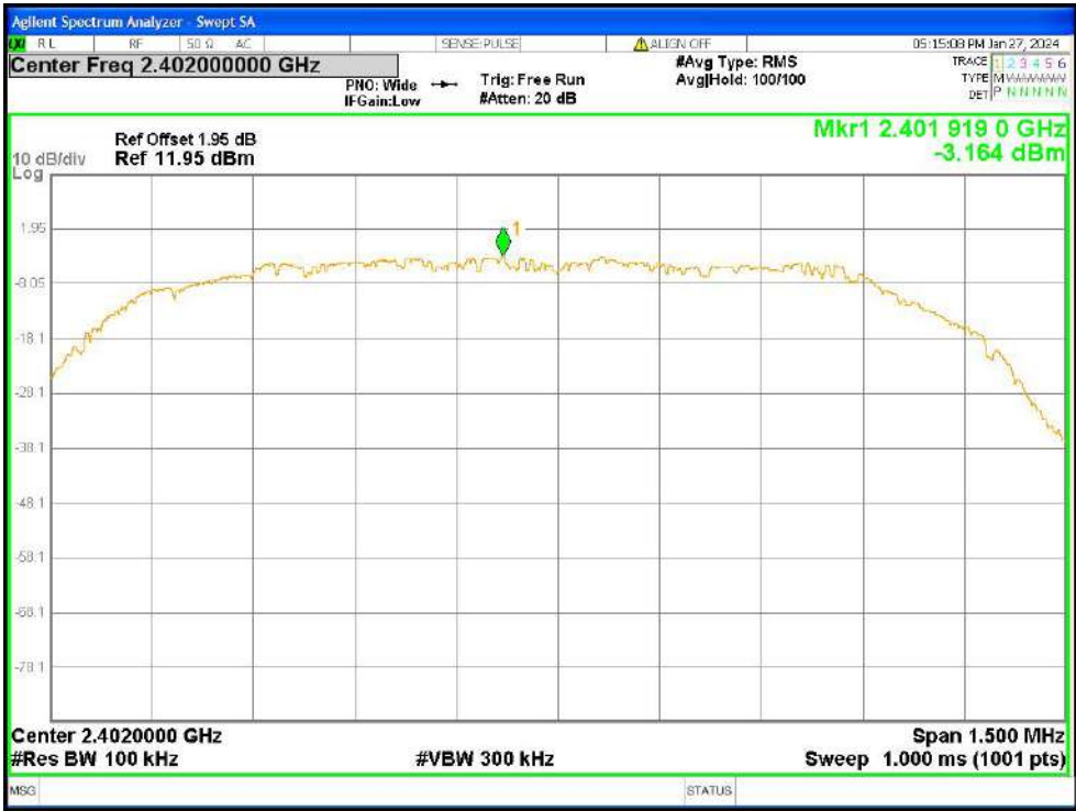
Tx. Spurious NVNT 3-DH5 2402MHz Ant1 Ref
