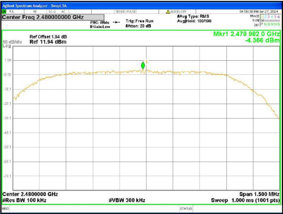
Tx. Spurious NVNT 2-DH5 2480MHz Ant1 Ref
