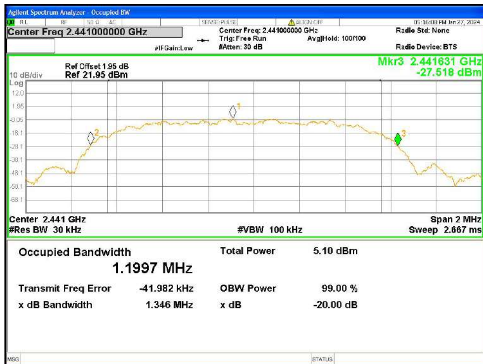
-20dB Bandwidth NVNT 3-DH5 2441MHz Ant1
