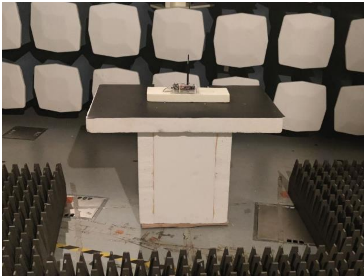
Picture 14, Radiated Spurious Emissions, EUT setup, RX 1 – 12,75 GHz
