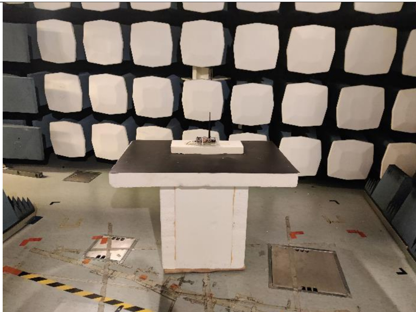
Picture 12, Radiated Spurious Emissions, EUT setup, TX and RX 30 – 1000 MHz
