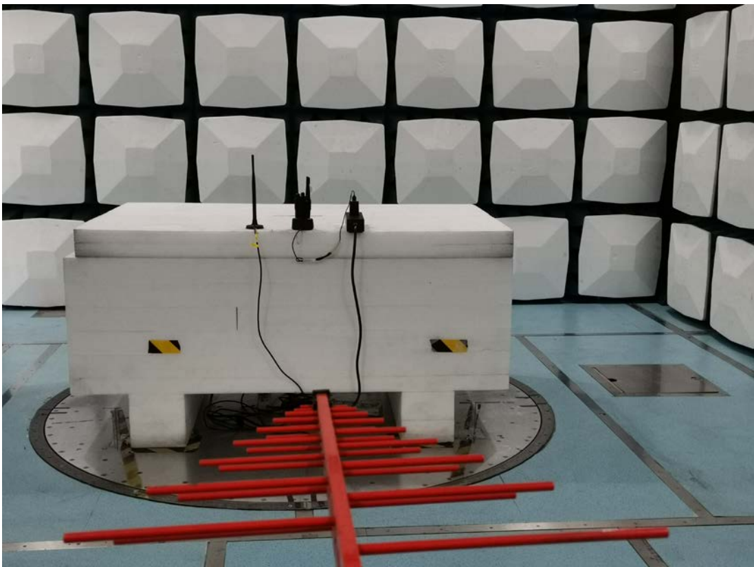
Radiated Emission Below 1GHz Rear View
