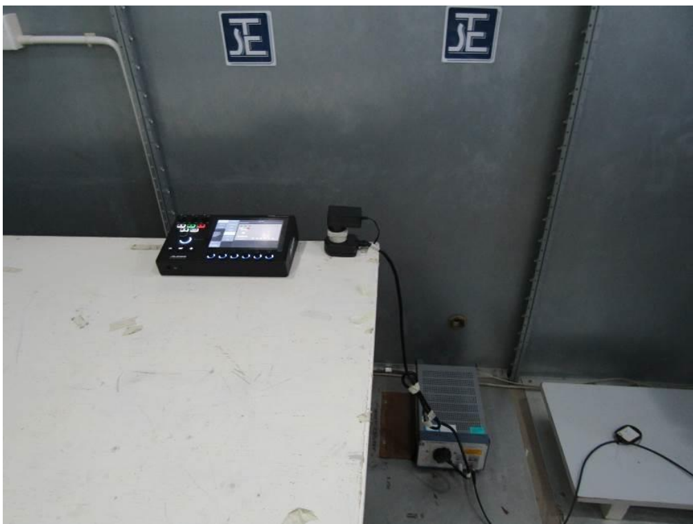
Measurement of Conducted Emission Test Set Up
