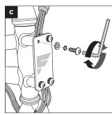
Note: Following installation of the front logo plate, check that the cables and wires can move freely by turning the handlebars fully to either side. If any resistance occurs, the wires and cables should be repositioned by sliding them up or down along the headtube.
