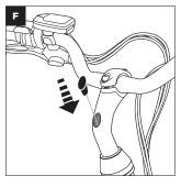
Note: Complete assembly of the bike per the steps below. The stem and handlebar angle can be adjusted as needed based on rider preference. Always re-tighten bolts to the specified torque values prior to riding.
