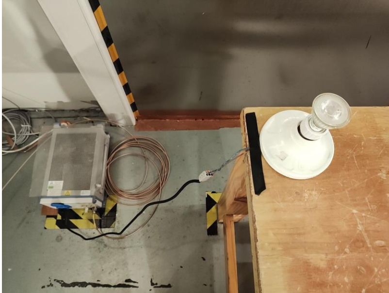
Photograph 2: Set-up for measurement of radiated emission
