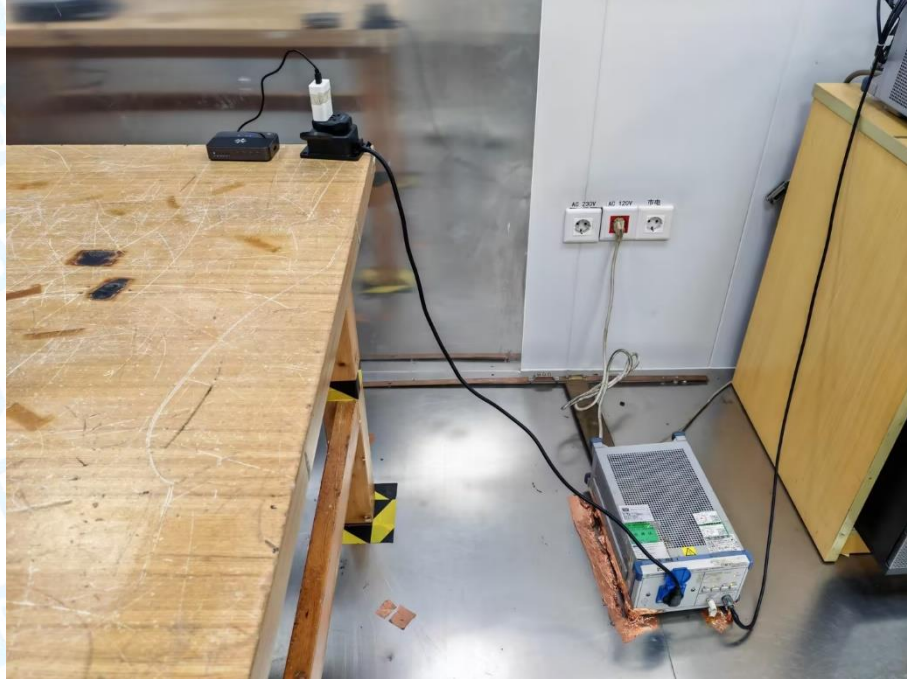
Photo of Setup for Radiated Emission (30MHz~1GHz)
