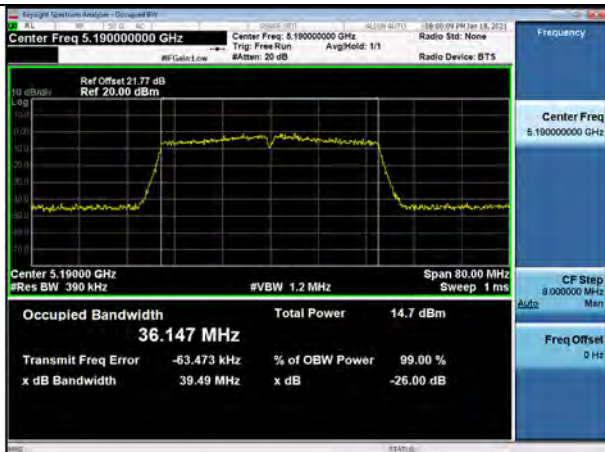
802.11ac_VHT40 UNII 2C BAND 26dB Bandwidth(CH 142)
