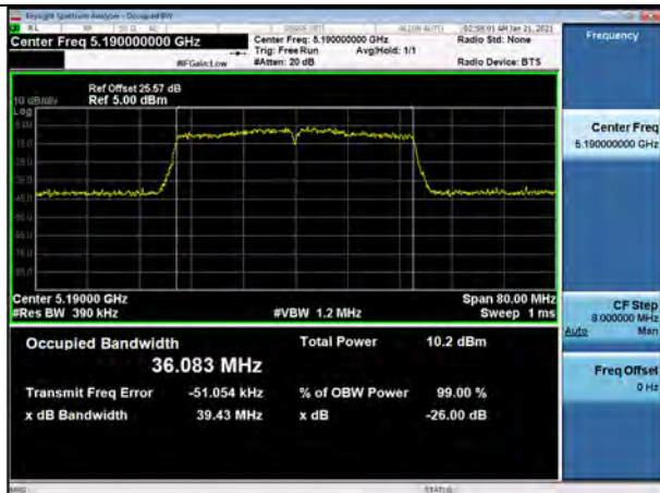
802.11ac_VHT40 UNII 2C BAND 26dB Bandwidth(CH 142)
