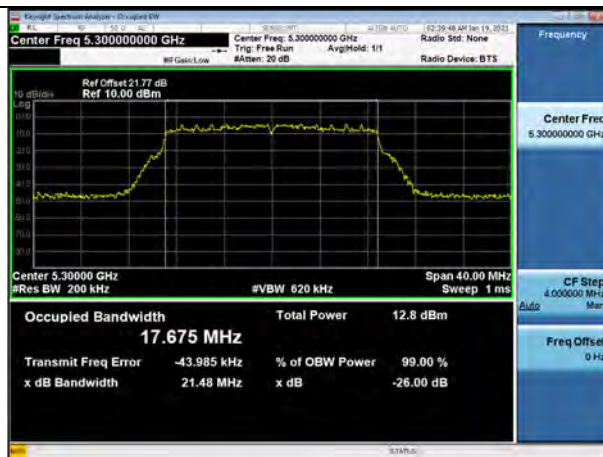
802.11n_HT20 UNII 3 BAND 26dB Bandwidth(CH 157)
