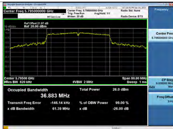
802.11n_HT40 UNII 3 BAND 26dB Bandwidth (CH 159)
