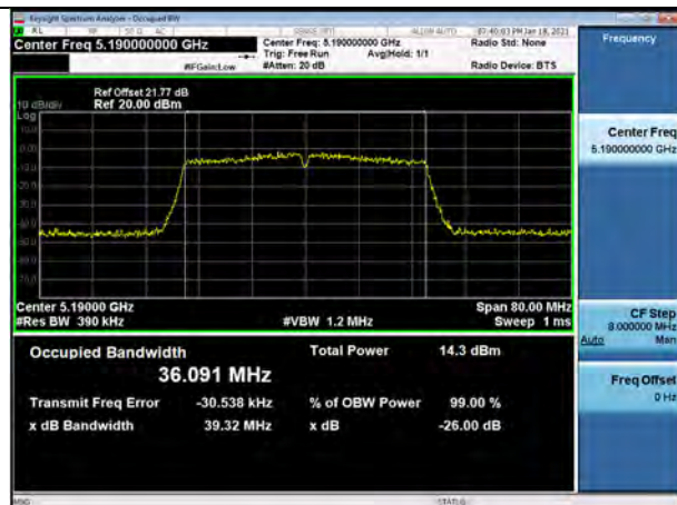
802.11n_HT40 UNII 2C BAND 26dB Bandwidth(CH 142)
