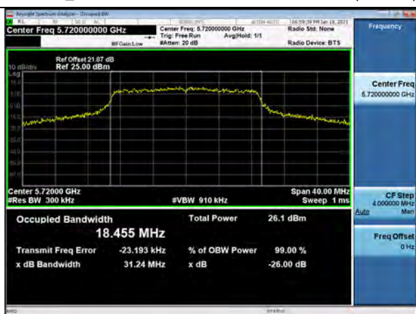
802.11n_HT20 UNII 2C BAND 26dB Bandwidth(CH 144)
