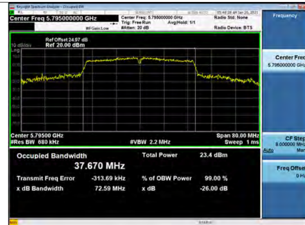
802.11ac_VHT40 UNII 3 BAND 26dB Bandwidth (CH 159)
