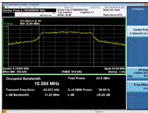
802.11n_HT20 UNII 3 BAND 26dB Bandwidth(CH 157)
