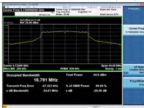
802.11a UNII 2C BAND 26dB Bandwidth (CH144)
