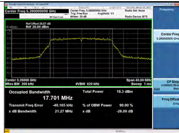
802.11ac_VHT20 UNII 3 BAND 26dB Bandwidth(CH 165)
