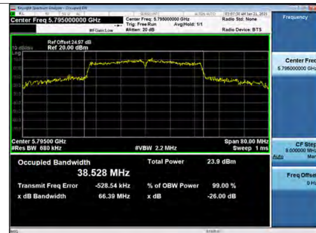
802.11ac_VHT40 UNII 3 BAND 26dB Bandwidth (CH 159)
