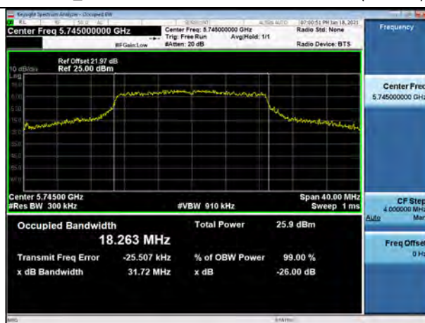
802.11n_HT20 UNII 3 BAND 26dB Bandwidth(CH 149)
