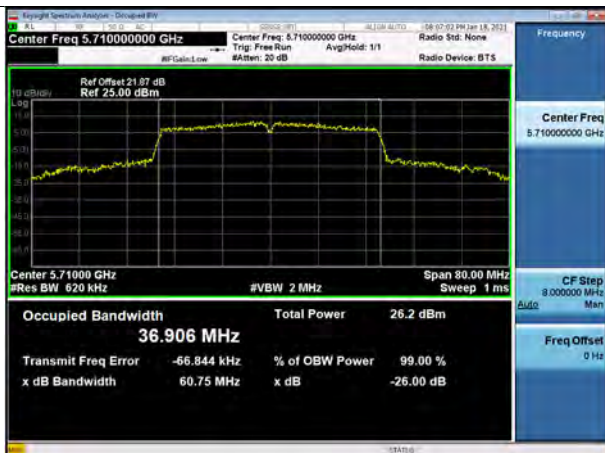
802.11ac_VHT40 UNII 2C BAND 26dB Bandwidth(CH 142)
