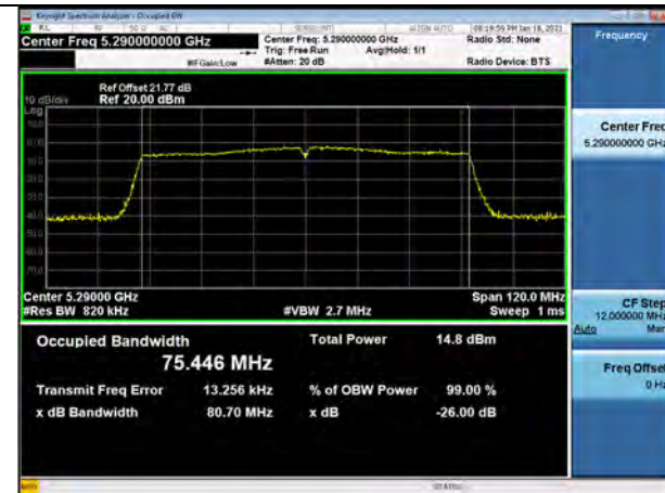
802.11ac_VHT80 UNII 3 BAND 26dB Bandwidth (CH 155)
