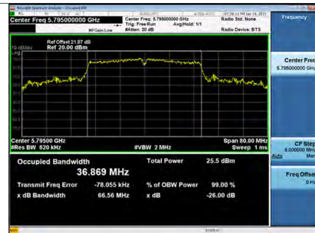
802.11ac_VHT40 UNII 3 BAND 26dB Bandwidth (CH 159)
