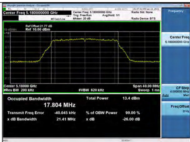
802.11n_HT20 UNII 2C BAND 26dB Bandwidth(CH 144)
