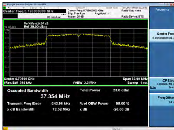
802.11n_HT40 UNII 3 BAND 26dB Bandwidth (CH 159)
