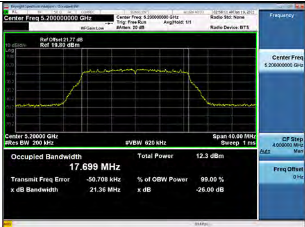
802.11ac_VHT20 UNII 2C BAND 26dB Bandwidth(CH 116)
