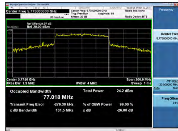
802.11ac_VHT80 UNII 3 BAND 26dB Bandwidth (CH 155)
