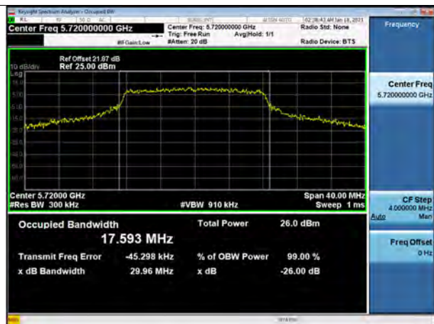
802.11a UNII 2C BAND 26dB Bandwidth (CH144)
