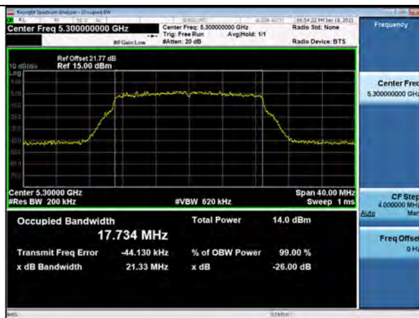
802.11n_HT20 UNII 3 BAND 26dB Bandwidth(CH 149)
