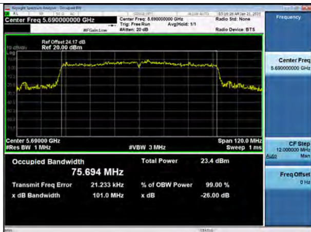
802.11ac_VHT80 UNII 2C BAND 26dB Bandwidth(CH 138)
