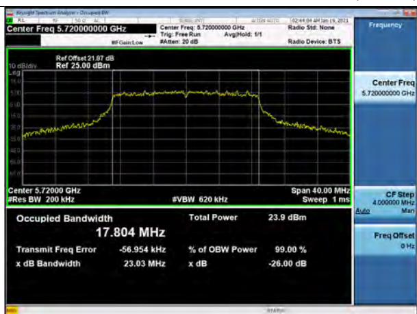
802.11n_HT20 UNII 2C BAND 26dB Bandwidth(CH 144)
