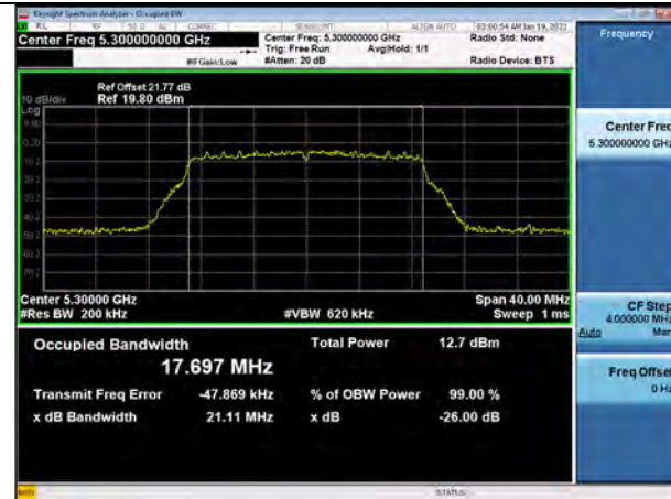
802.11ac_VHT20 UNII 3 BAND 26dB Bandwidth(CH 157)
