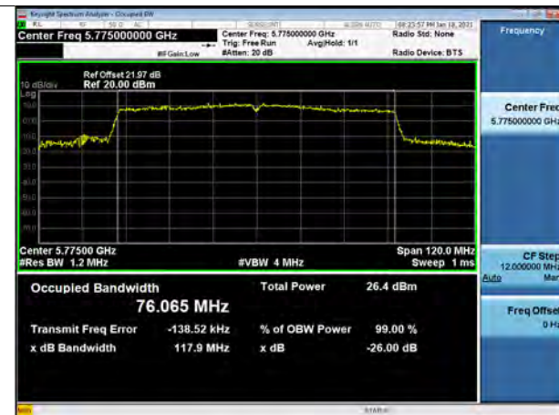
802.11ac_VHT80 UNII 3 BAND 26dB Bandwidth (CH 155)
