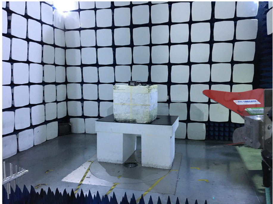
Radiation Emission Test Setup (1GHz to 18GHz)
