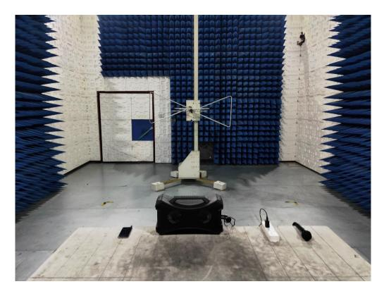
RADIATED EMISSION TEST SETUP ABOVE 1GHZ
