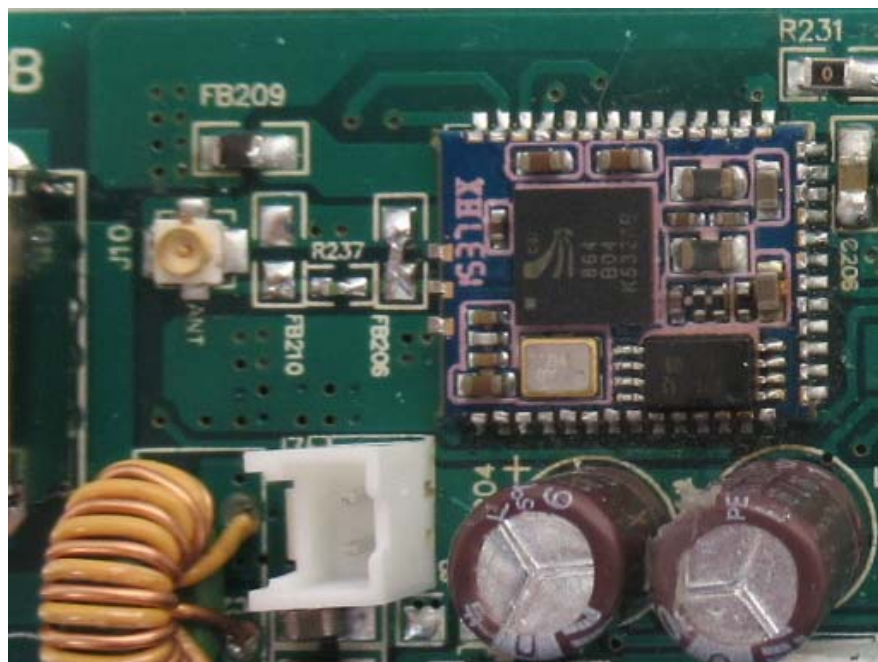
EUT- BT3.0 Module View
