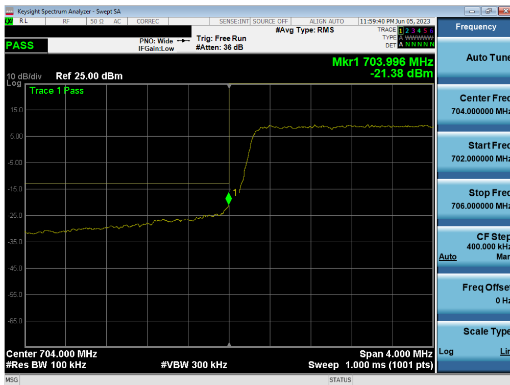
Plot 7-112. Lower Band Edge Plot (LTE Band 17 - 5MHz QPSK – Full RB)
