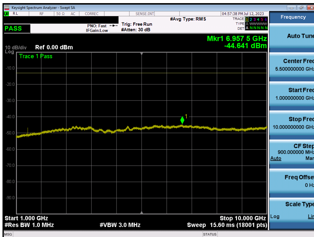
Plot 7-40. Conducted Spurious Plot (LTE Band 12/17 - 10MHz QPSK - RB Size 1, RB Offset 0 - Mid Channel)
