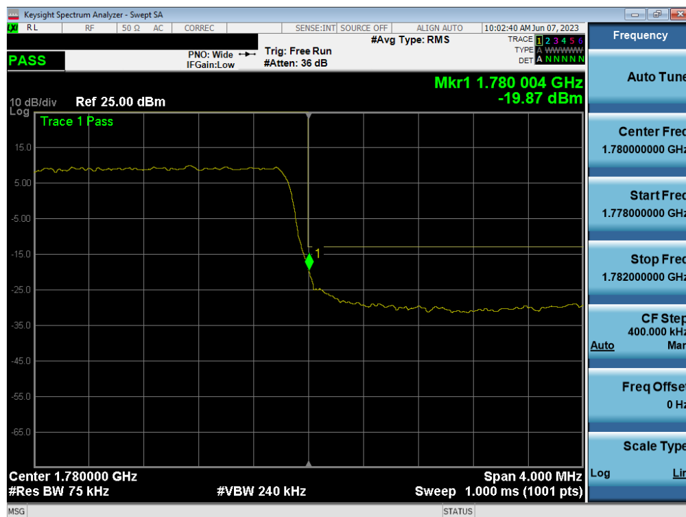
Plot 7-62. Upper Band Edge Plot (LTE Band 66 - 3MHz QPSK – Full RB)
