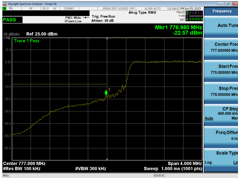
Plot 7-120. Lower Band Edge Plot (LTE Band 13 - 10MHz QPSK – Full RB)
