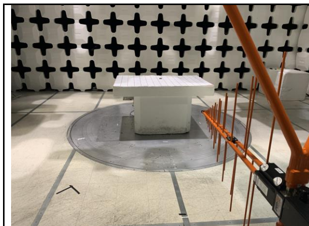
Radiated Emission Test below 1GHz Front View
