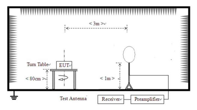
2) For radiated emissions from 30MHz to1GHz
