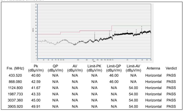
(433.92MHz, Antenna Horizontal, 30MHz to 5GHz)
