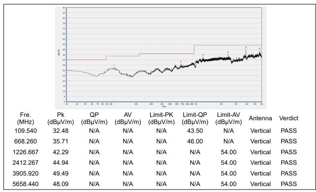
(433.92MHz, Antenna Vertical, 30MHz to 5GHz)
