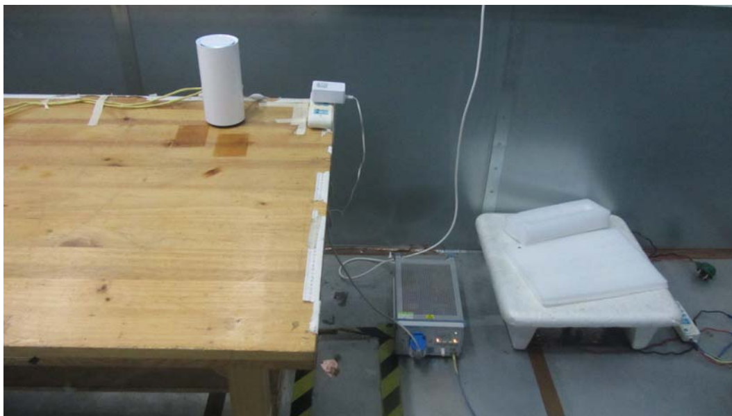
Picture 3 Conducted Emission Test Setup
