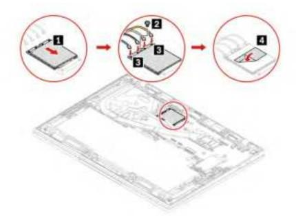
**Note:** During installation, ensure that you connect the cables with different colors to the corresponding connectors on the card according to the illustrations above: the orange cable to the connector labeled ORANGE, the blue cable to the connector labeled BLUE, the white and grey cable to the connector labeled WHITE GREY, and the black and grey cable to the connector labeled BLACK GREY.
