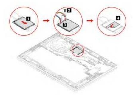
**Note:** During installation, ensure that you connect the cables with different colors to the corresponding connectors on the card according to the illustrations above: the orange cable to the connector labeled ORANGE, the blue cable to the connector labeled BLUE.
