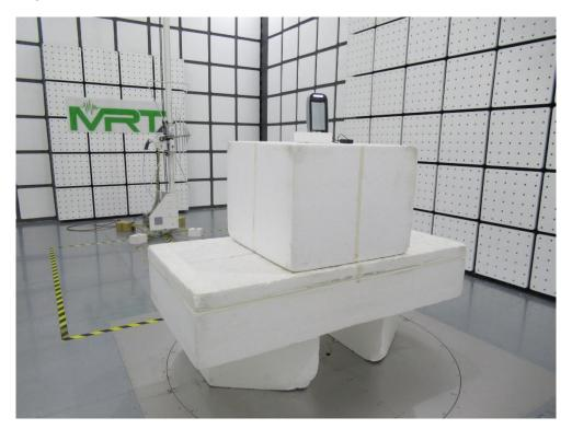
Description: Radiated Emission Test Setup Monarch 8 inch (BUTTERFLYMX.M08) for Above 1GHz
