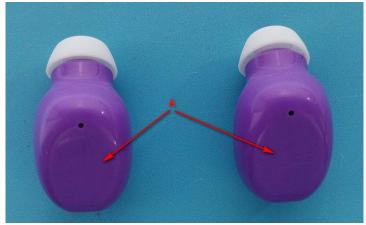
B. Top cover (B): The plastic logo of the top cover does not provide enough physical space to fit the printing of the FCC ID according to below reference picture.
