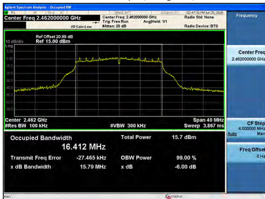
6dB Bandwidth plot (802.11g-CH 11)
