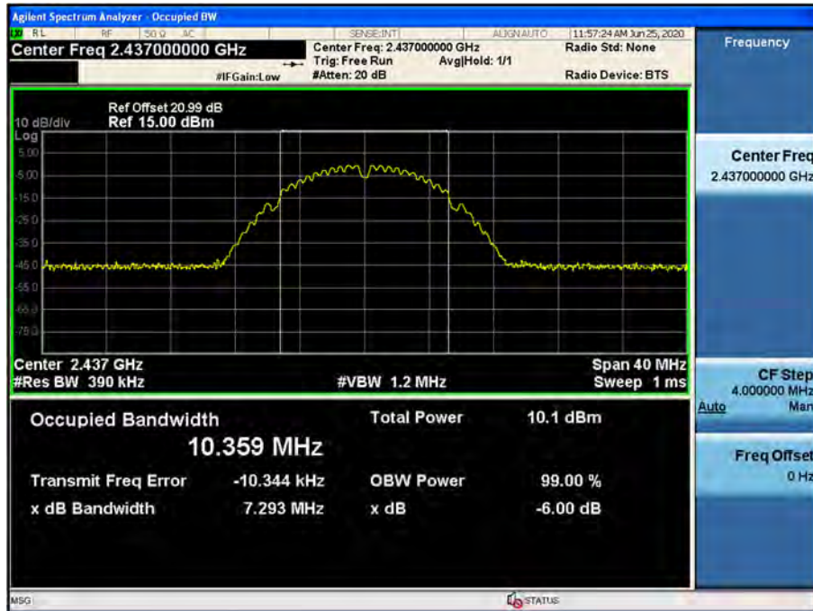
99% Bandwidth plot (802.11b-CH 6)
