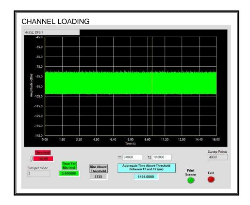
The level of traffic loading on the channel by the EUT is 14.94%.
