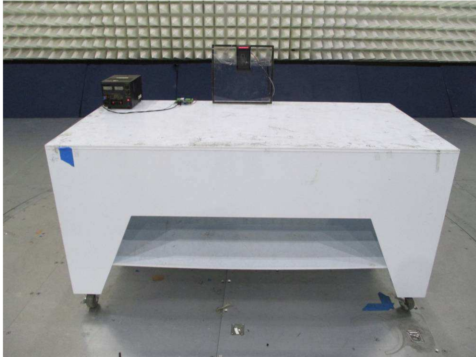
Radiated Emission test above 30 MHz
