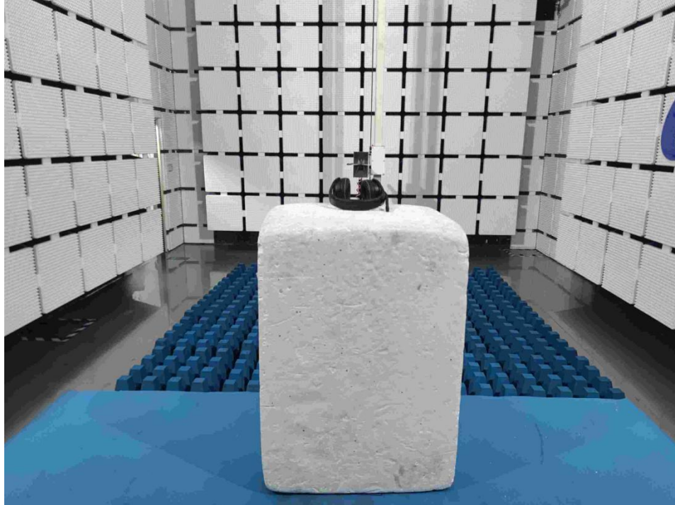
Radiated Emissions (above 1GHz)
