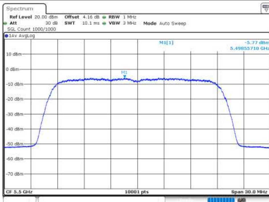
PSD NVNT ax20 5500MHz Ant2
