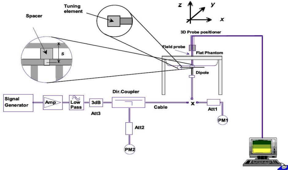
The output power on dipole port must be calibrated to 20 dBm (100mW) before dipole is connected.
