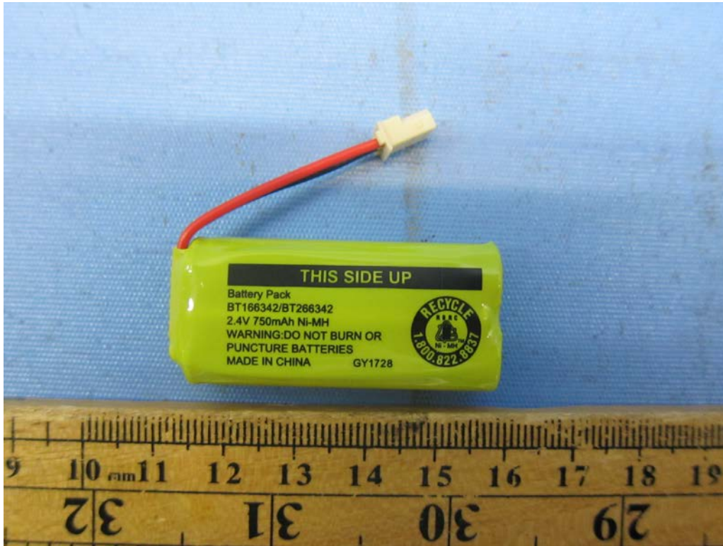
Figure 3 - 2.4V 750mAh Coslight Ni-MH rechargeable battery
