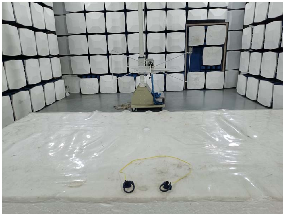
Radiated emission test view
