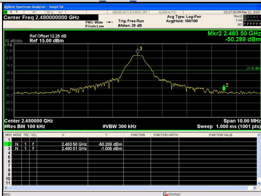
Out Of Band Emission GFSK DH5 Channel 78
