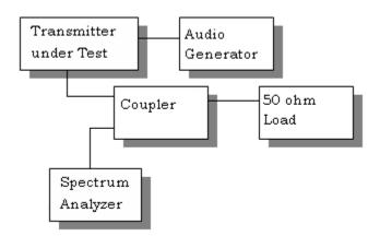
**Antenna Conducted Emissions:** The RBW = 100 kHz, VBW = 300 kHz and the span set to 10.0 MHz and the spectrum was scanned from 30 MHz to the  $10^{th}$  Harmonic of the fundamental. Above 1 GHz the resolution bandwidth was 1 MHz and the VBW = 3 MHz and the span to 50 MHz.
