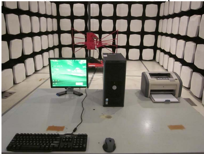
Measurement of Radiated Emission Test Set Up
