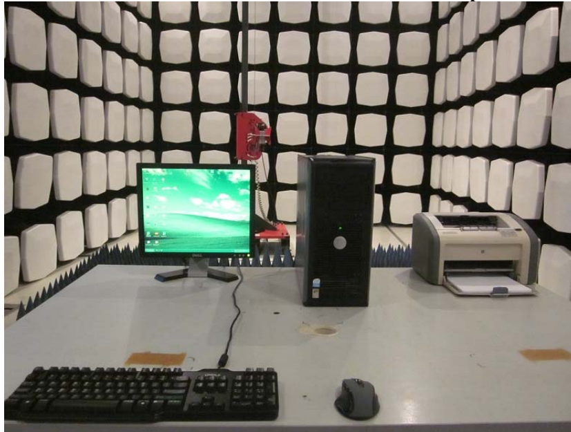
Measurement of Radiated Emission Test Set Up
