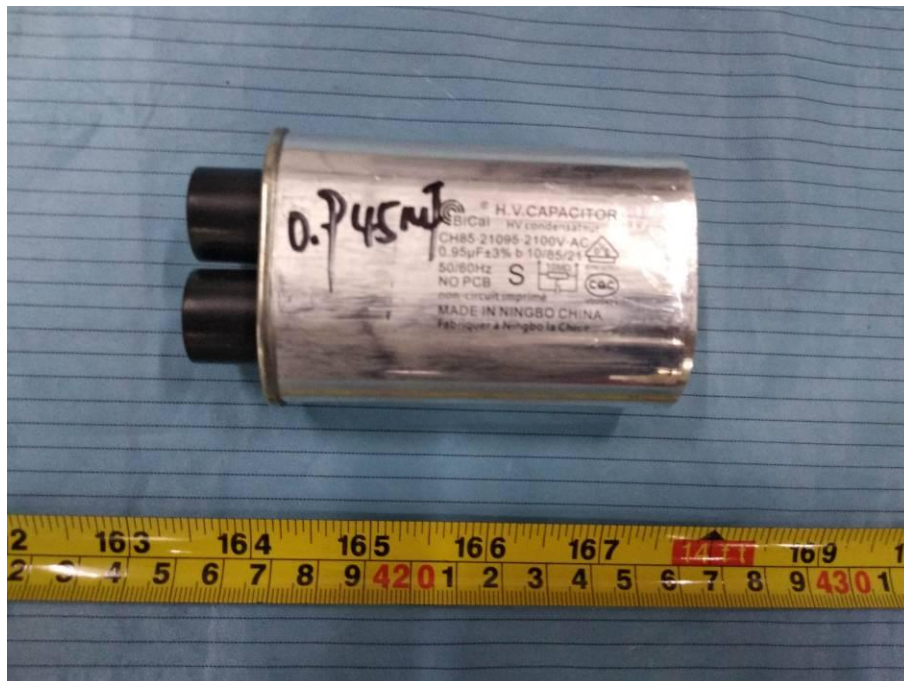
EUT – H.V. Capacitor Front View
