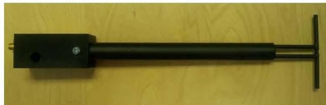
Figure 1 – MVG COMOSAR Validation Dipole
