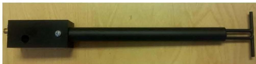
Figure 1 – MVG COMOSAR Validation Dipole
