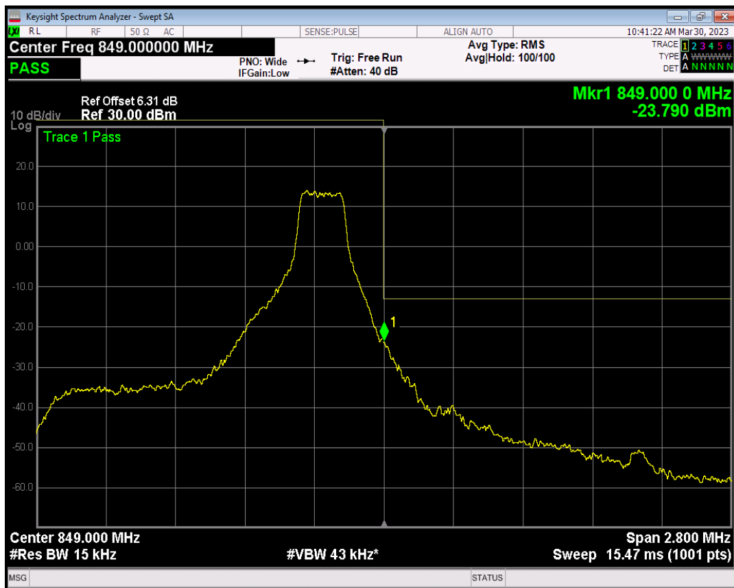
Band5 QPSK BW=1.4MHz Channel=20643 RB Size=6 Position=#0
