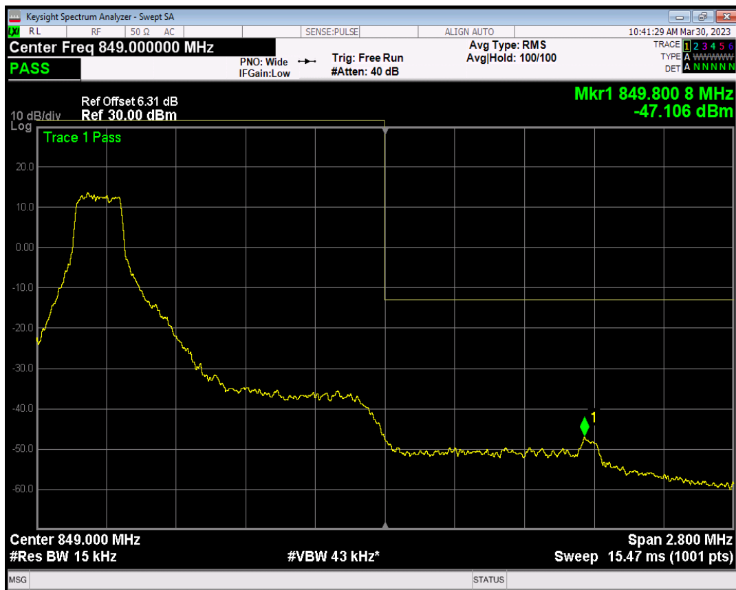
Band5 QAM16 BW=1.4MHz Channel=20643 RB Size=1 Position=#Max
