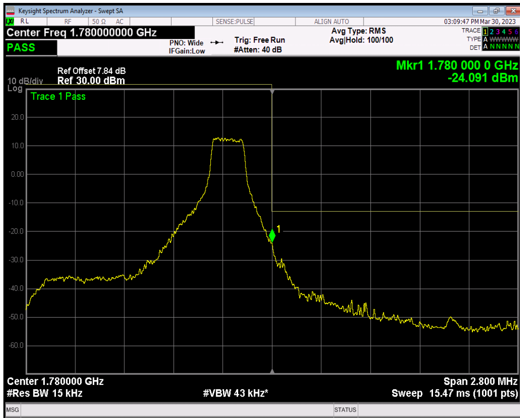
Band66 QAM16 BW=1.4MHz Channel=132665 RB Size=6 Position=#0
