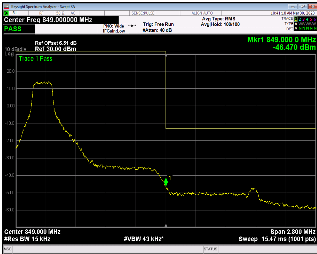
Band5 QPSK BW=1.4MHz Channel=20643 RB Size=1 Position=#Max
