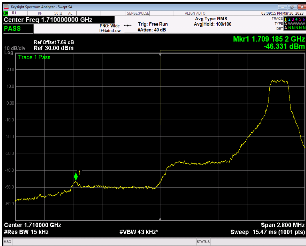
Band66 QPSK BW=1.4MHz Channel=131979 RB Size=6 Position=#0
