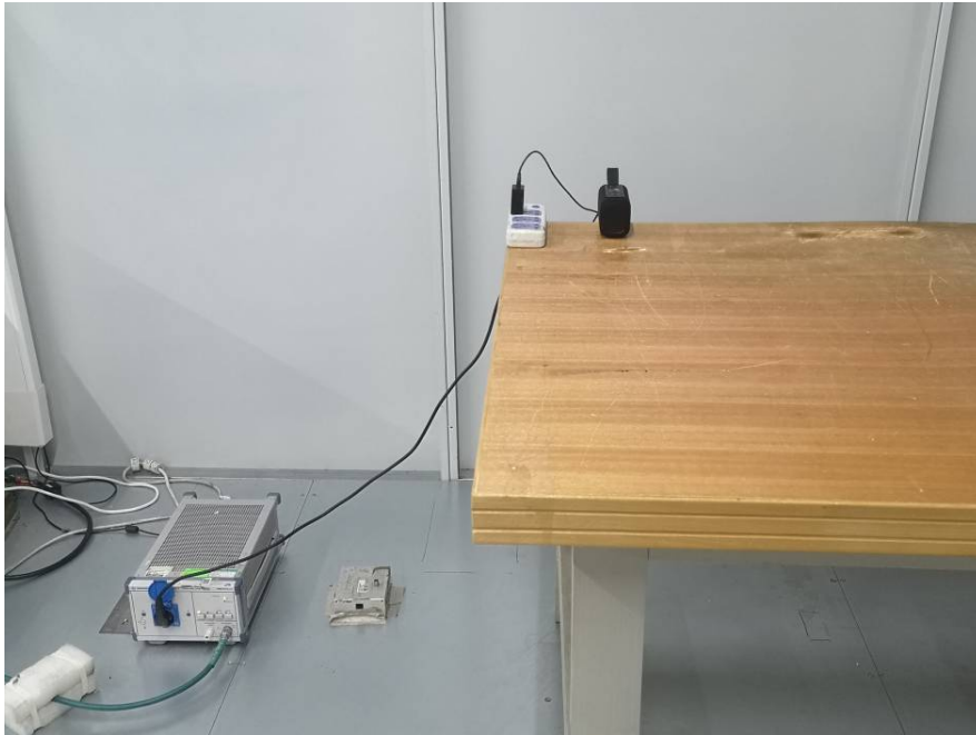
Conducted Emissions - Front View
