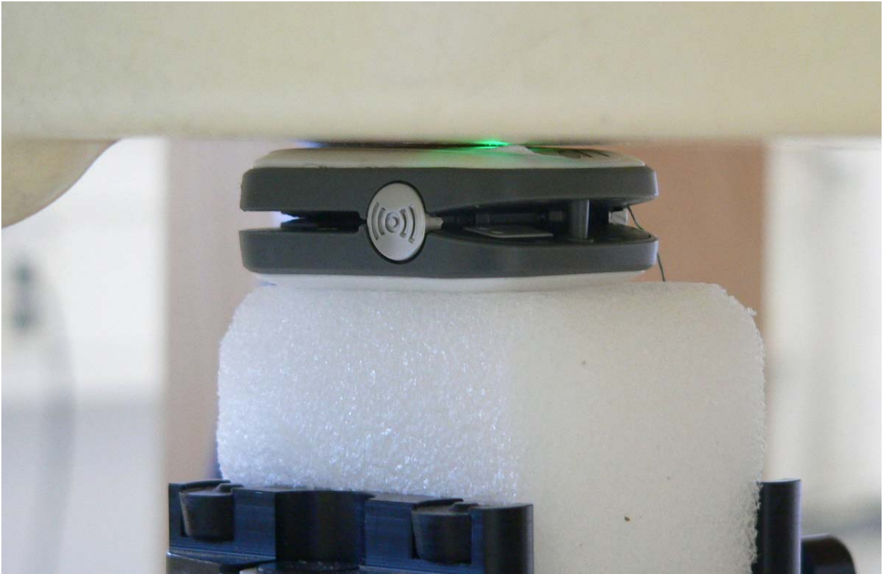
Fig. 17: GPRS 850/1900, top side of Buddi Click System - Clip, 0 mm gap.
