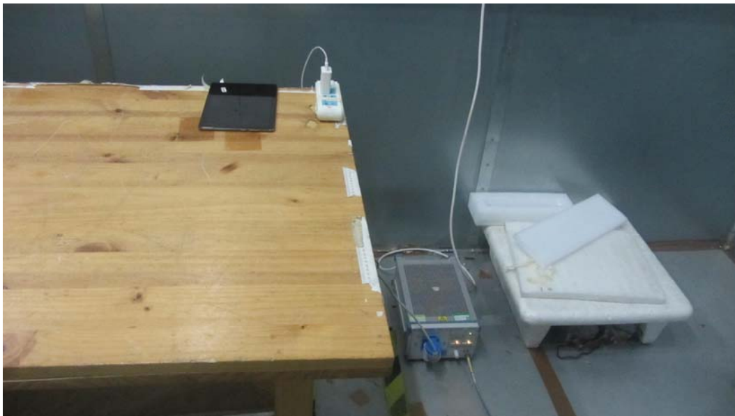
Picture 2 Conducted Emission Test Setup
