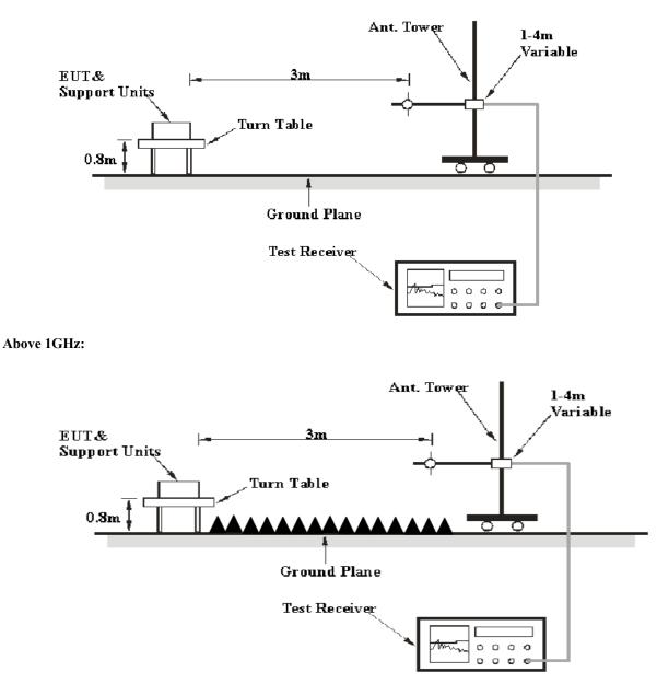
The radiated emission tests were performed in the 3 meters chamber test site, using the setup accordance with the ANSI C63.4-2014. The specification used was the FCC Part 15.109 Class B limits. Note: The distance is 1m when the radiated emission above 25GHz is investigated.
