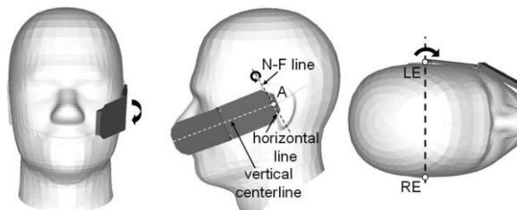
8. While keeping the handset in contact with the pinna, rotate the handset around a line perpendicular to the plane defined by the handset vertical centerline and horizontal line and passing through handset point A, until the handset vertical centerline is in the Reference Plane. Note that this step is necessary, as the handset may not be in the reference plane after step 7)
