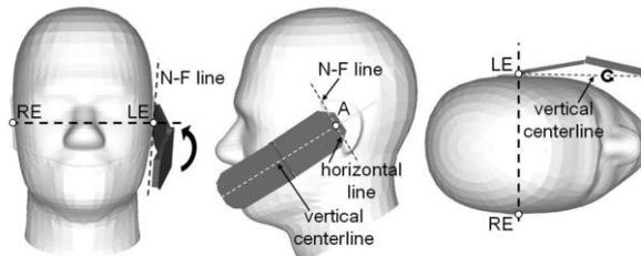
7. While keeping point A on the line passing through RE and LE, and maintaining the handset in contact with the pinna at the ERP, rotate the handset about the N-F line until any point on the handset is in contact with a phantom point below the pinna on the cheek
