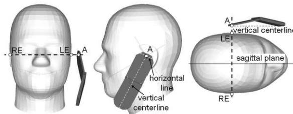
4. Translate the handset towards the phantom along the line passing through RE and LE until the handset touches the pinna
