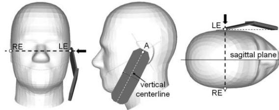
5. Rotate the handset around the (virtual) LE-RE line until the handset vertical centerline is in the Reference Plane
