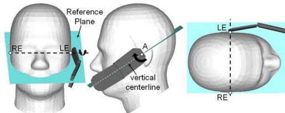
6. Rotate the handset around the vertical centerline until the plane defined by the handset vertical centerline and horizontal line is parallel to the N-F line, and translate the handset along the LE-RE line toward the phantom until handset touches the pinna
