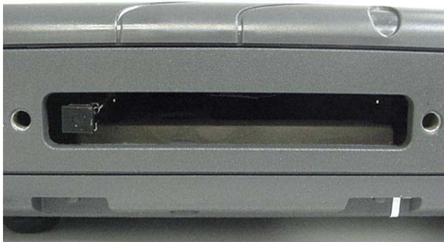
PCMCIA Slot (Hatch & AirCard 775 Removed)
