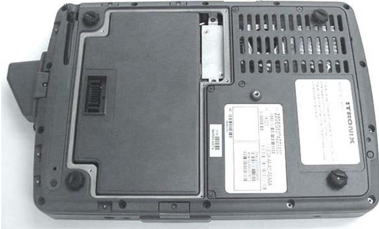
DUT with Internal Li-ion Battery 11.1 V, 3600 mAh (Model: T8M-E)
