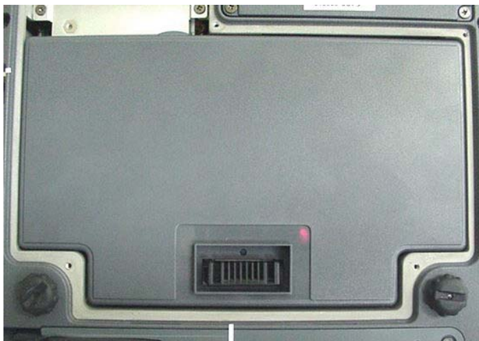
Internal Li-ion Battery 11.1 V, 3600 mAh (Model: T8M-E)
