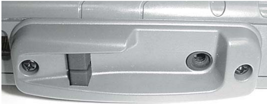
IX325 Hatch for AirCard 775 (Antenna Removed)
