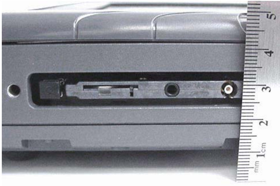
PCMCIA Slot-to-Base Distance (Hatch & Antenna Removed)
