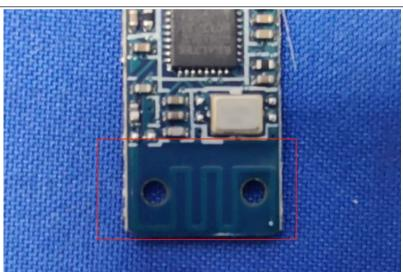
The antenna is PCB antenna.
