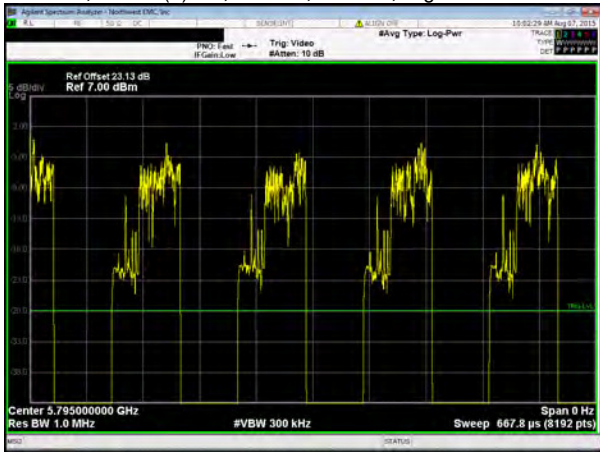
Chain B, 802.11(n) HT, MCS23, 40 MHz, High Channel 5795 MHz
