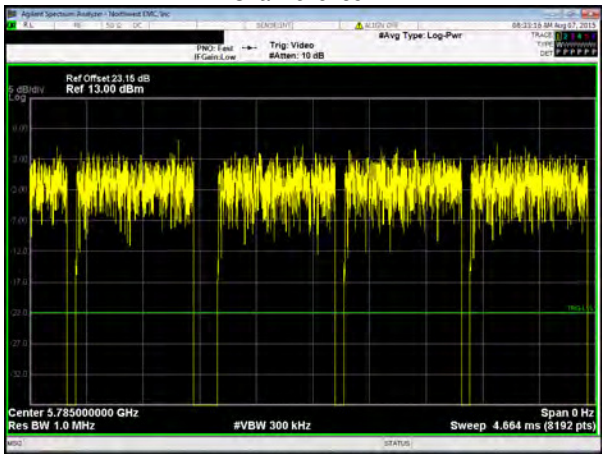
Chain B, 802.11(ac) VHT, MCS8 (256-QAM), 20 MHz, Mid Channel 5785 MHz
