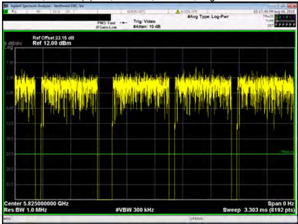
Chain A, 802.11(n) HT, MCS16, 20 MHz, High Channel 5825 MHz
