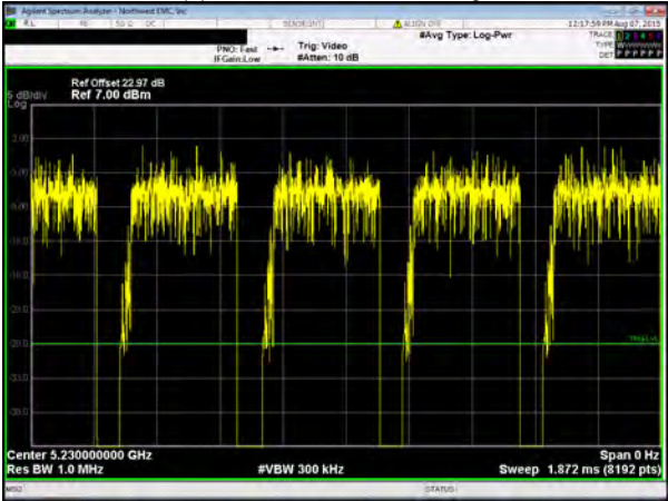
Chain C, 802.11(n) HT, MCS16, 40 MHz, High Channel 5230 MHz
