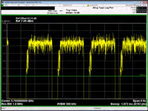
Chain A, 802.11(n) HT, MCS16, 40 MHz, High Channel 5795 MHz
