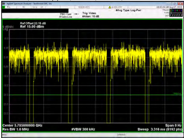
Chain B, 802.11(n) HT, MCS16, 20 MHz, Mid Channel 5785 MHz
