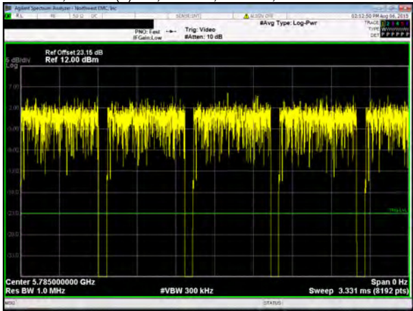
Chain A, 802.11(n) HT, MCS16, 20 MHz, Mid Channel 5785 MHz
