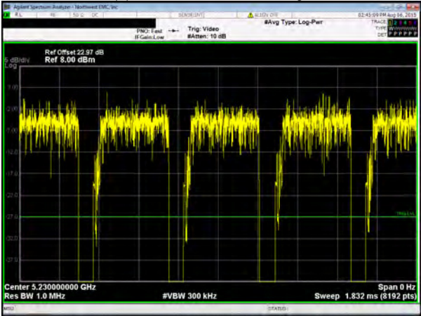
Chain A, 802.11(n) HT, MCS16, 40 MHz, High Channel 5230 MHz
