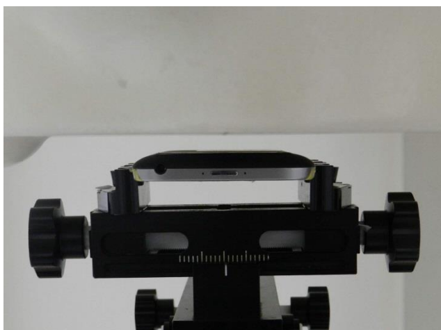
Back, Test Separation 1 cm
