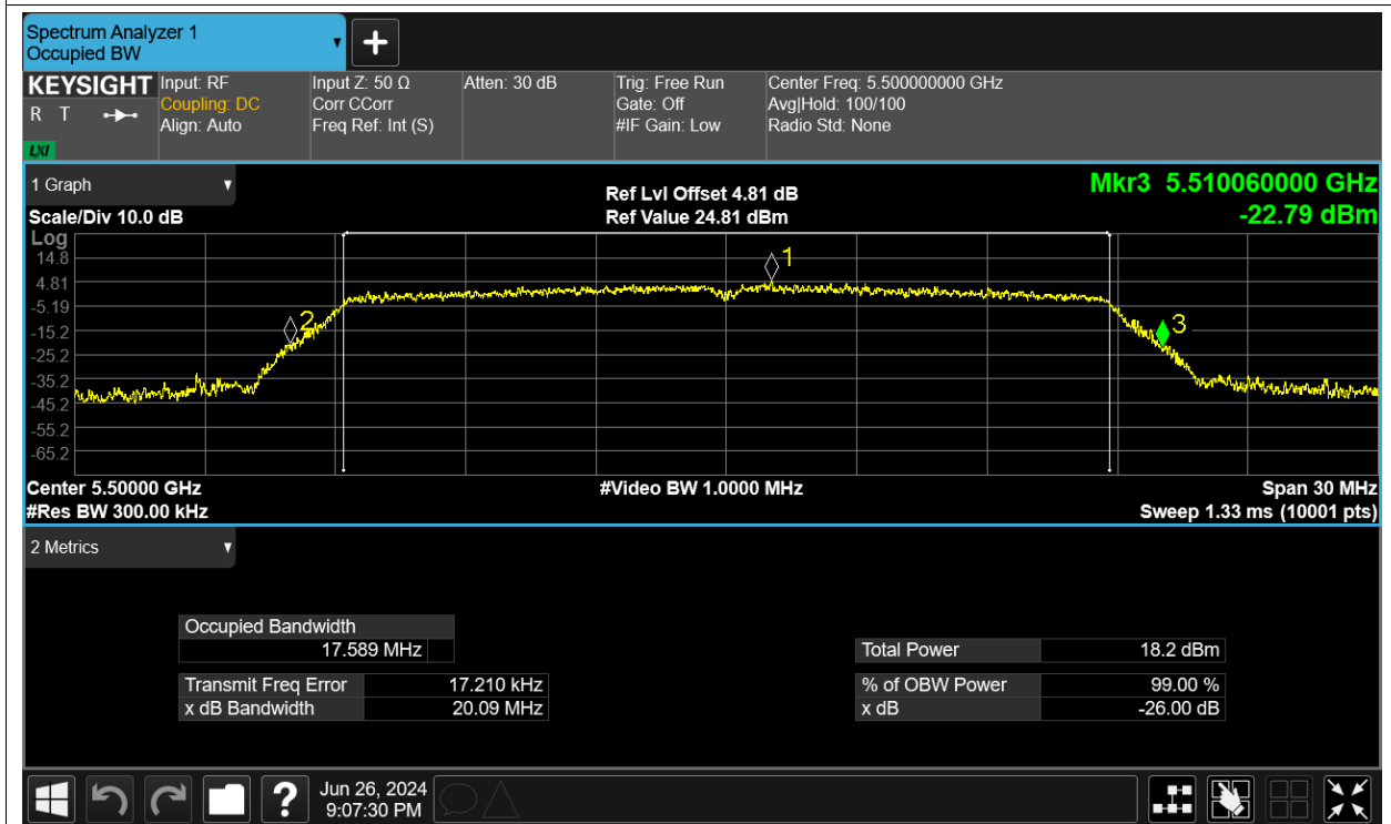
-26dB Bandwidth NVNT n20 5600MHz Ant1
