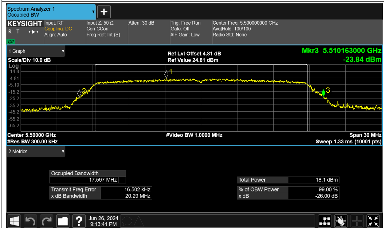
-26dB Bandwidth NVNT ac20 5600MHz Ant1
