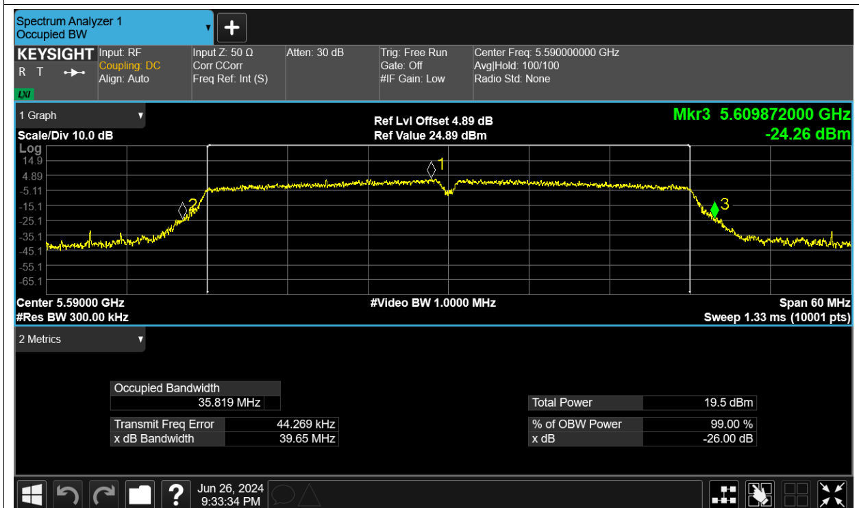
-26dB Bandwidth NVNT ac40 5670MHz Ant1
