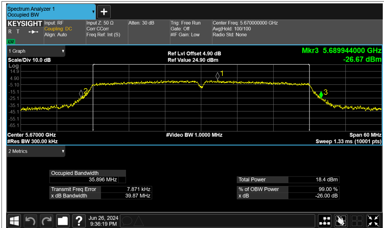
-26dB Bandwidth NVNT ac80 5530MHz Ant1
