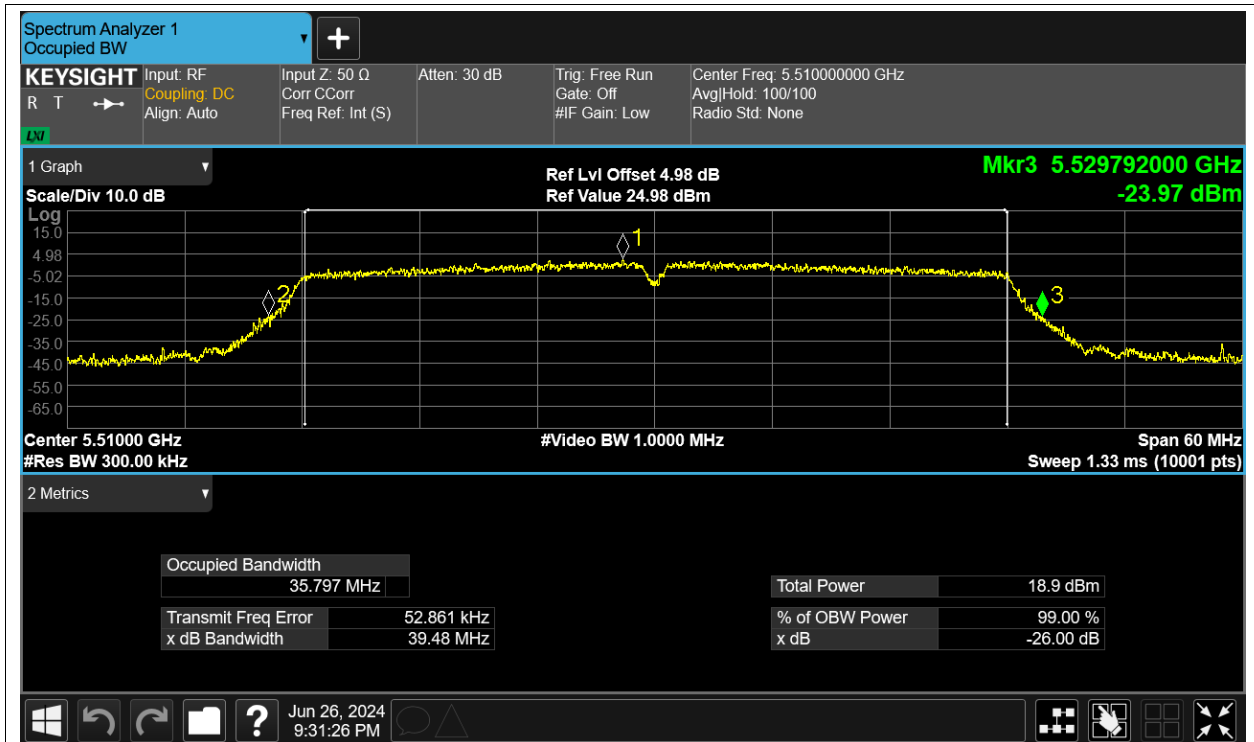
-26dB Bandwidth NVNT ac40 5590MHz Ant1
