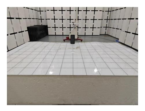
**Set-up for Radiated Spurious Emission, Above 1GHz**
