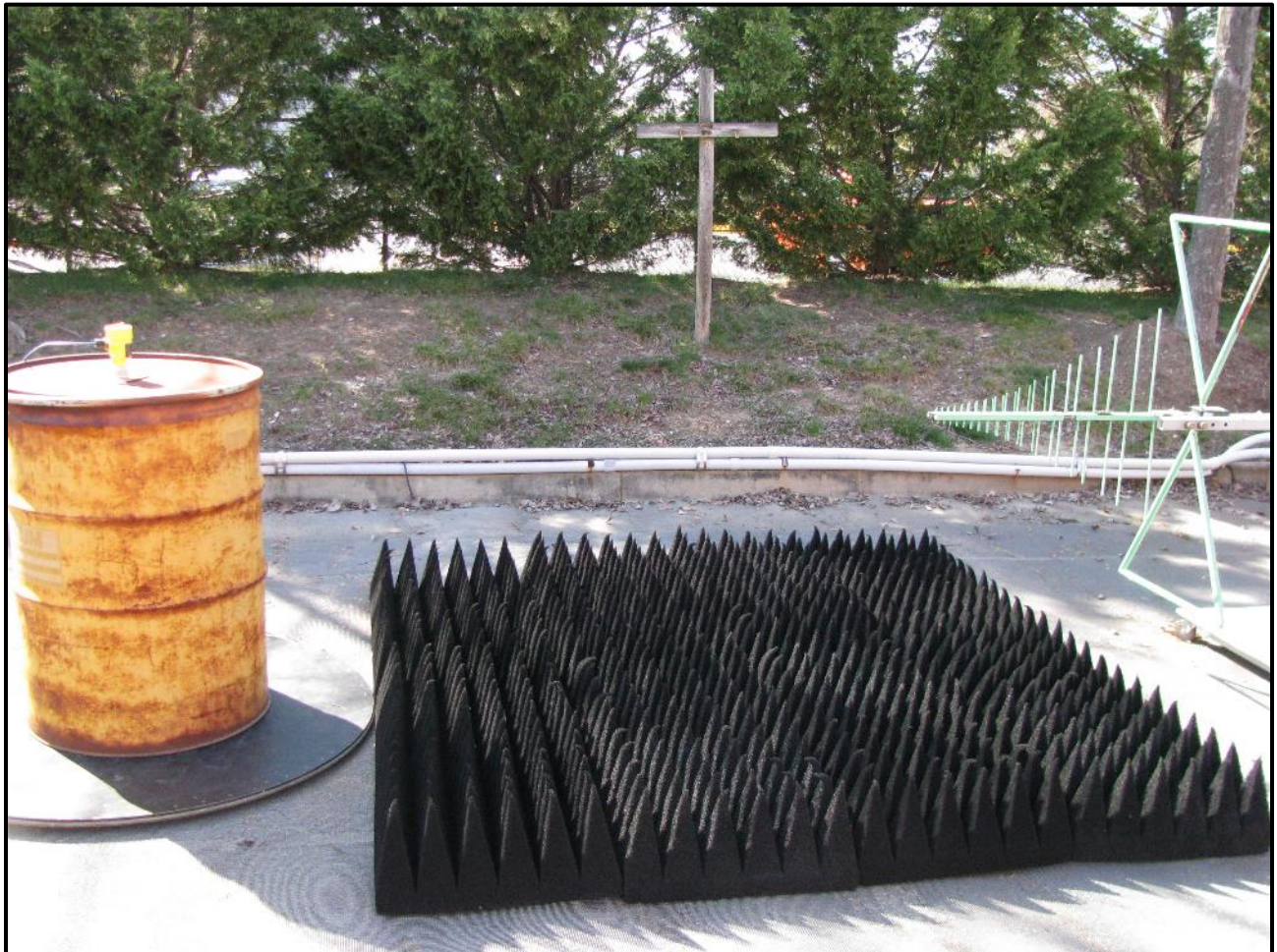
Photograph 23: Radiated Emissions – TC #6; Steel Container, Front View
