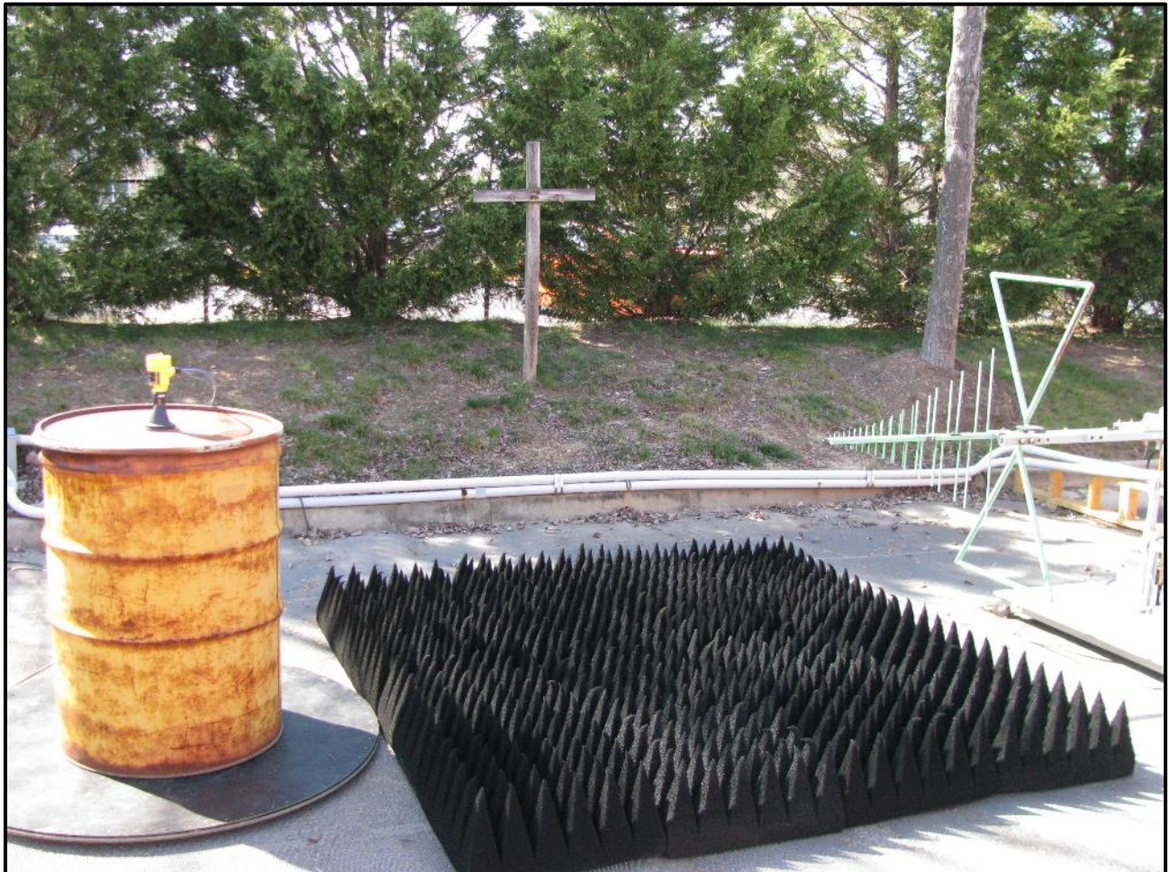
Photograph 14: Radiated Emissions – TC #1; Steel Container, Rear View
