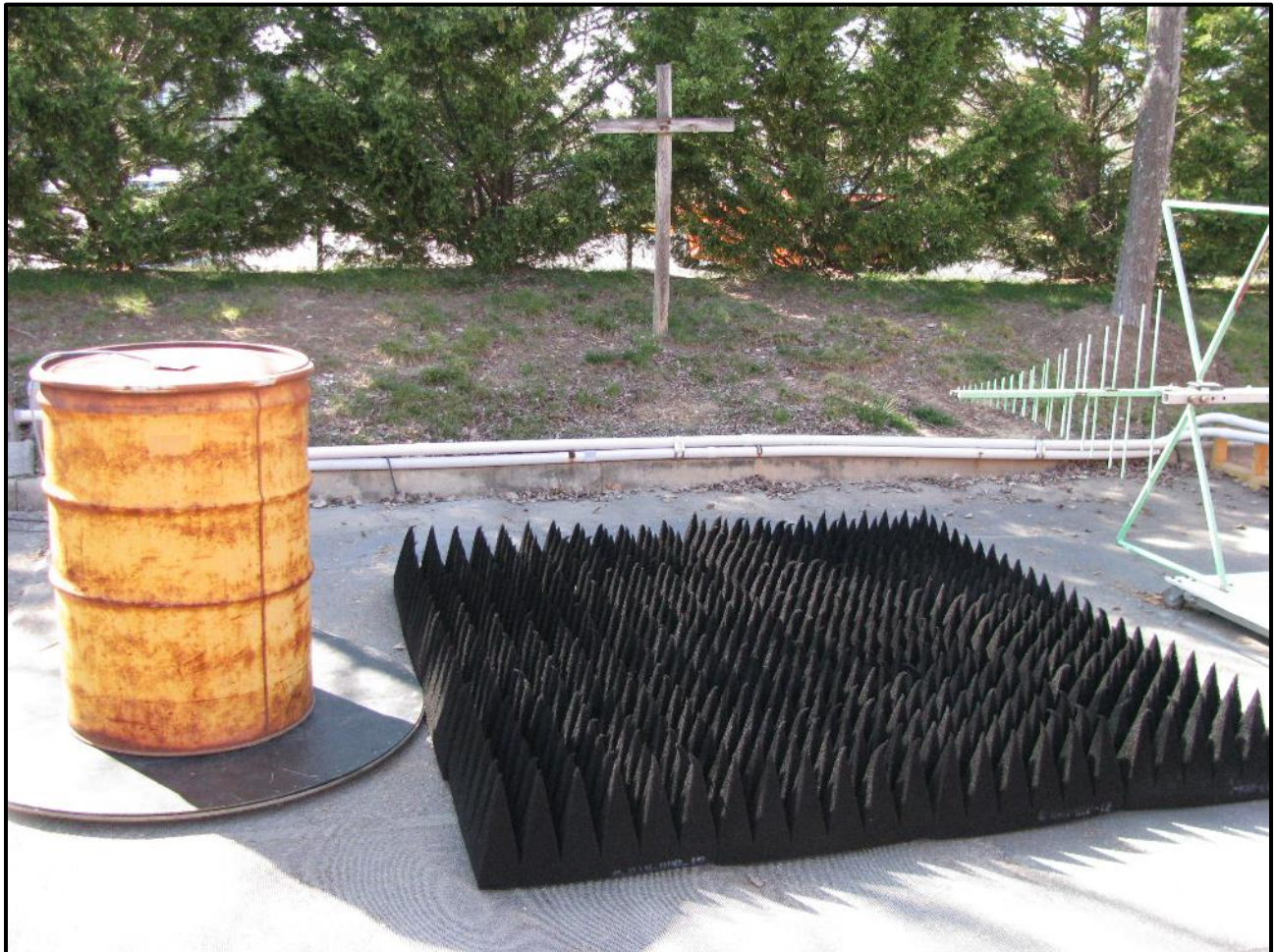
Photograph 27: Radiated Emissions – TC #8; Steel Container, Front View
