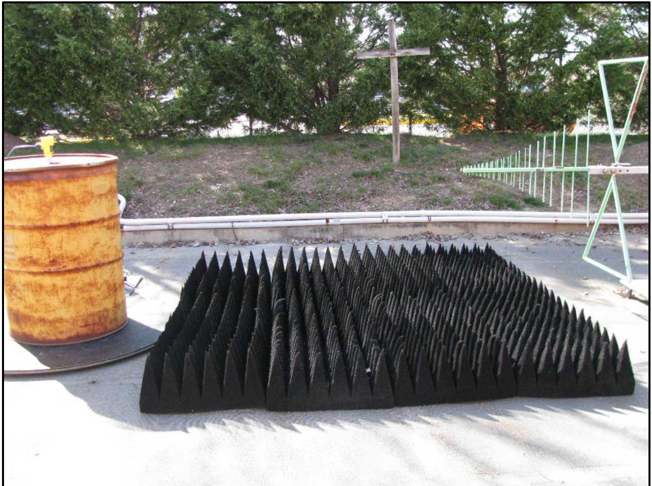
Photograph 24: Radiated Emissions – TC #6; Steel Container, Rear View
