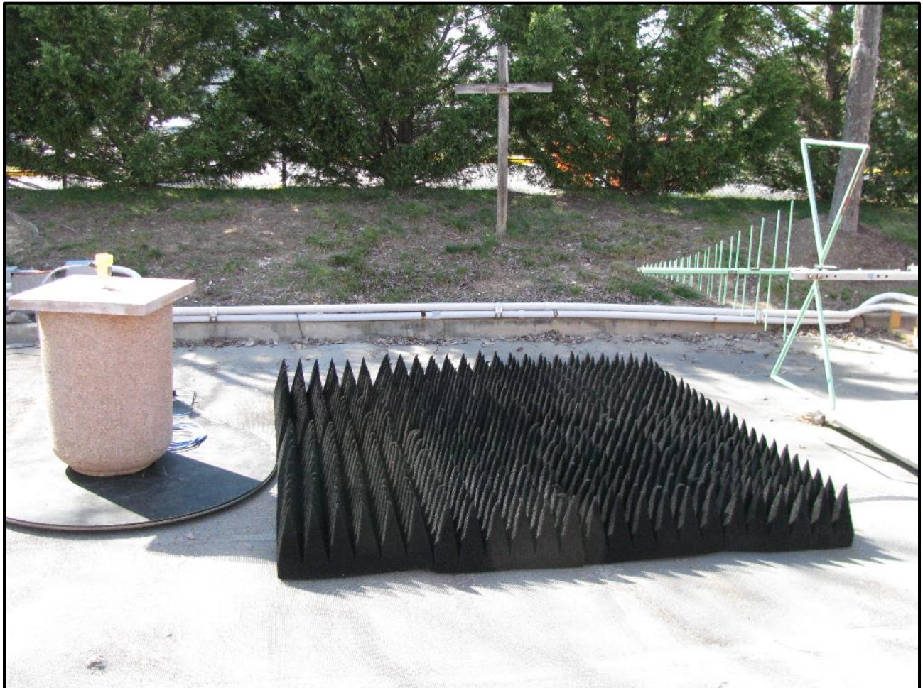
Photograph 38: Radiated Emissions – TC #4; Concrete Container, Rear View
