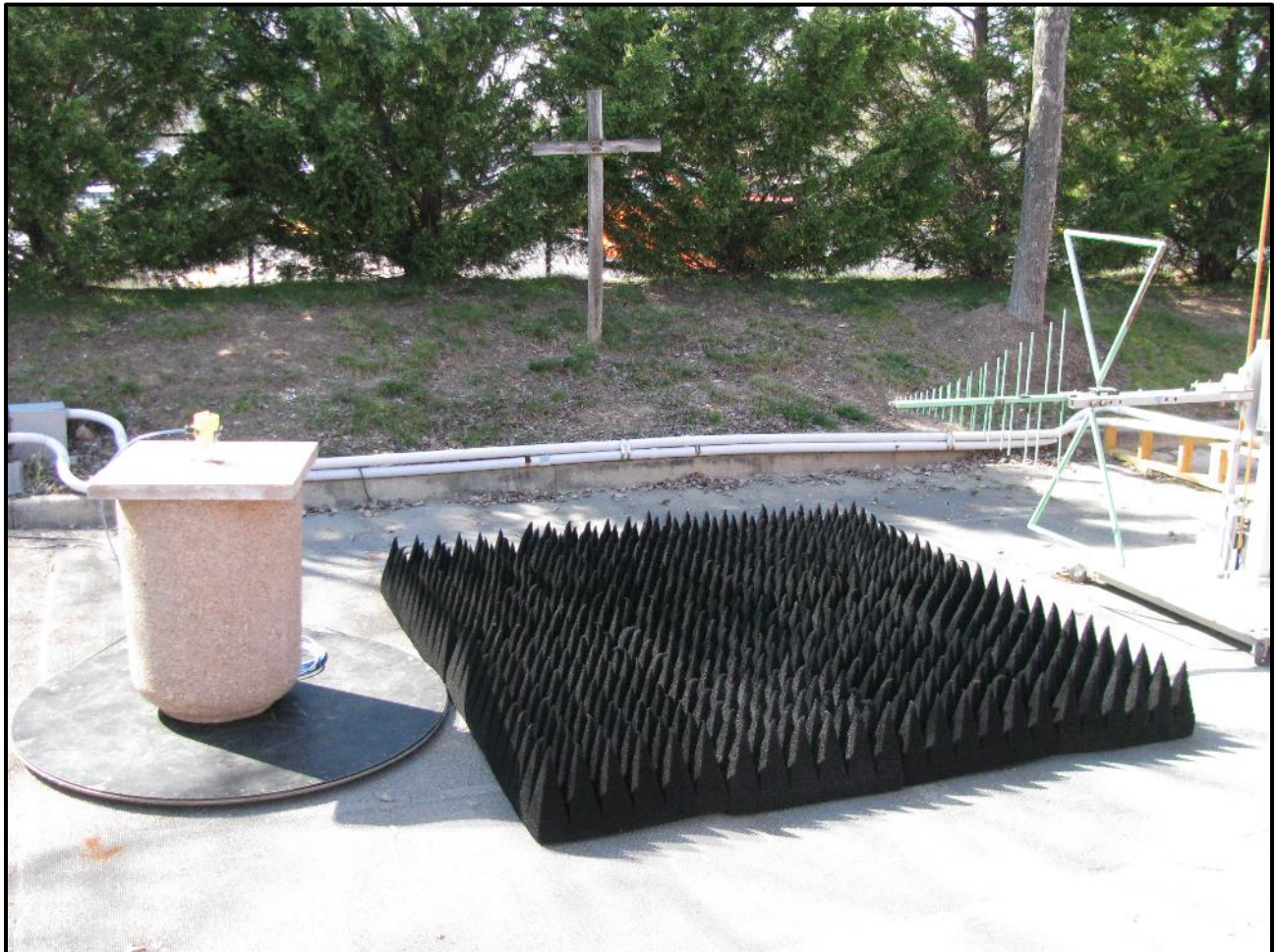
Photograph 42: Radiated Emissions – TC #6; Concrete Container, Rear View
