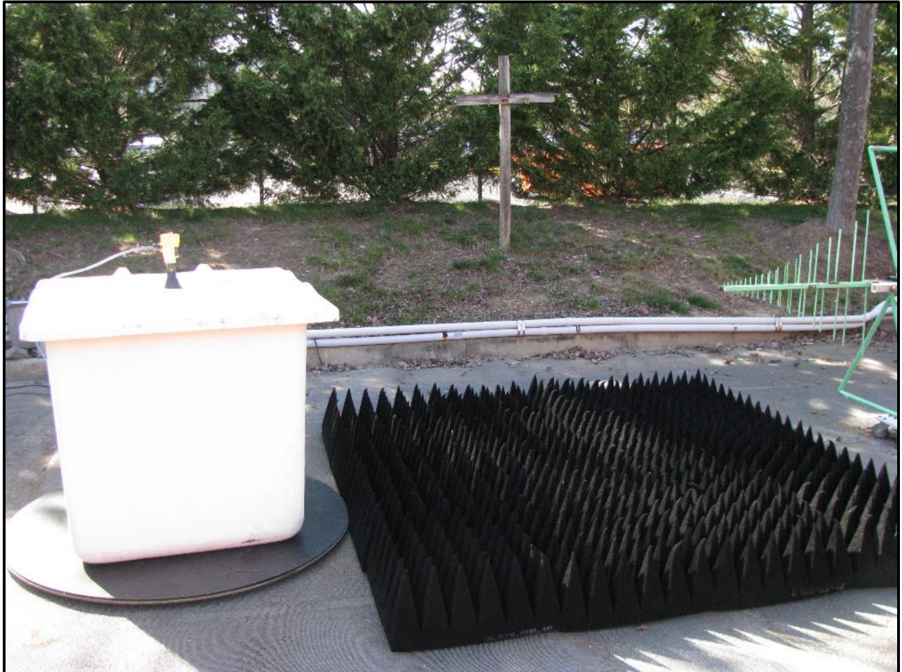
Photograph 49: Radiated Emissions – TC #1; Fiberglass Container, Front View
