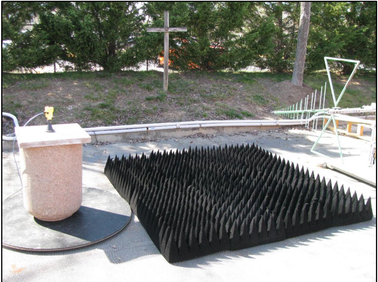
Photograph 32: Radiated Emissions – TC #1; Concrete Container, Rear View
