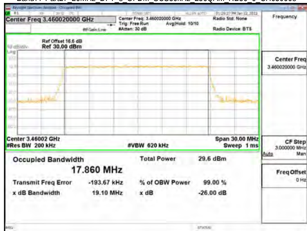
Band77-Part27 20MHz DFT s OFDM SCS30kHz 256QAM RB50 0 CH633334
