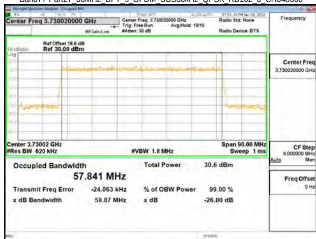
Band77-Part27 60MHz DFT s OFDM SCS30kHz QPSK RB162 0 CH648668
