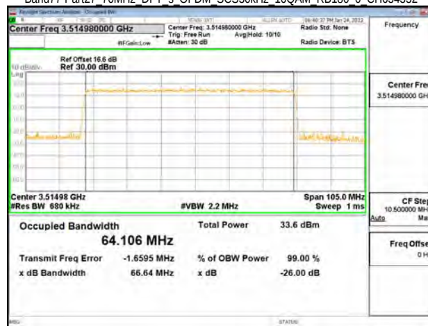
Band77-Part27 70MHz DFT s OFDM SCS30kHz 16QAM RB180 0 CH634332
