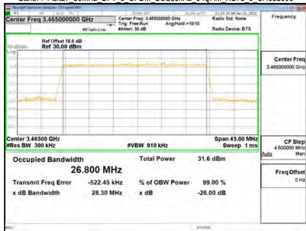
Band77-Part27 30MHz DFT s OFDM SCS30kHz 64QAM RB75 0 CH633334
