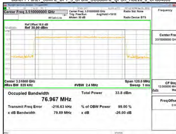
Band77-Part27 80MHz DFT s OFDM SCS30kHz QPSK RB216 0 CH634000
