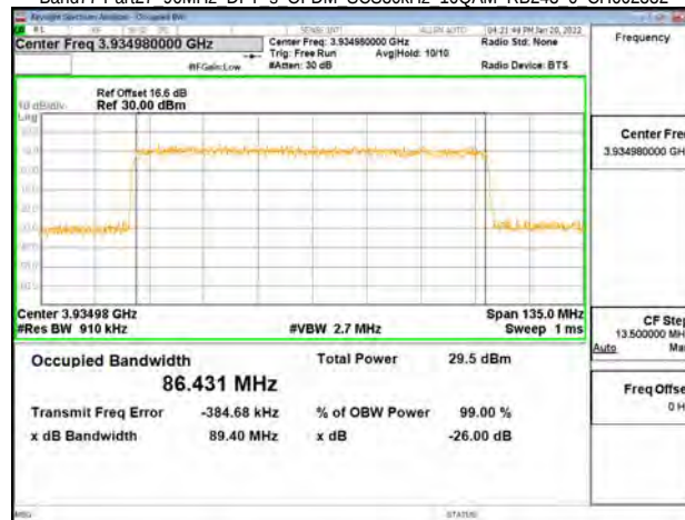
Band77-Part27 90MHz DFT s OFDM SCS30kHz 64QAM RB243 0 CH649668
