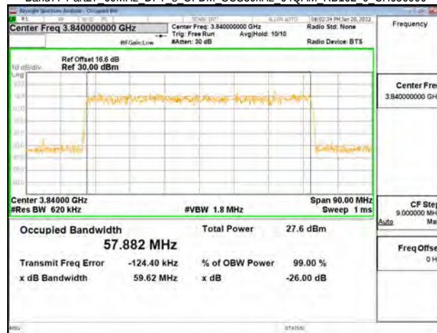
Band77-Part27 60MHz DFT s OFDM SCS30kHz 64QAM RB162 0 CH663332
