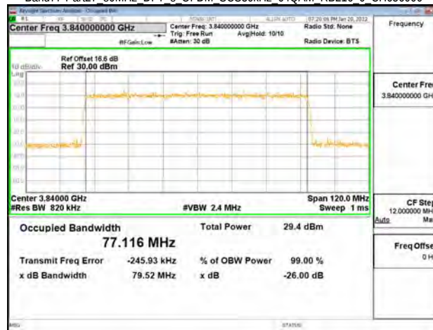
Band77-Part27 80MHz DFT s OFDM SCS30kHz 64QAM RB216 0 CH662666
