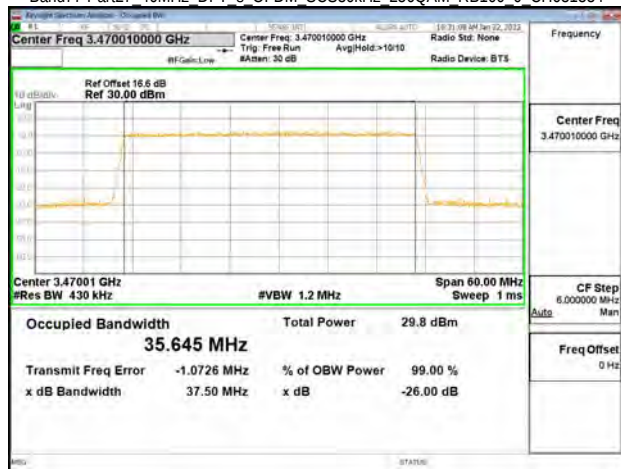
Band77-Part27 40MHz DFT s OFDM SCS30kHz 256QAM RB100 0 CH633334
