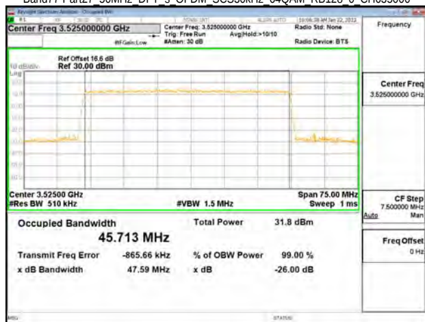
Band77-Part27 50MHz DFT s OFDM SCS30kHz 64QAM RB128 0 CH635000
