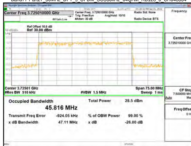
Band77-Part27 50MHz DFT s OFDM SCS30kHz 64QAM RB128 0 CH648334
