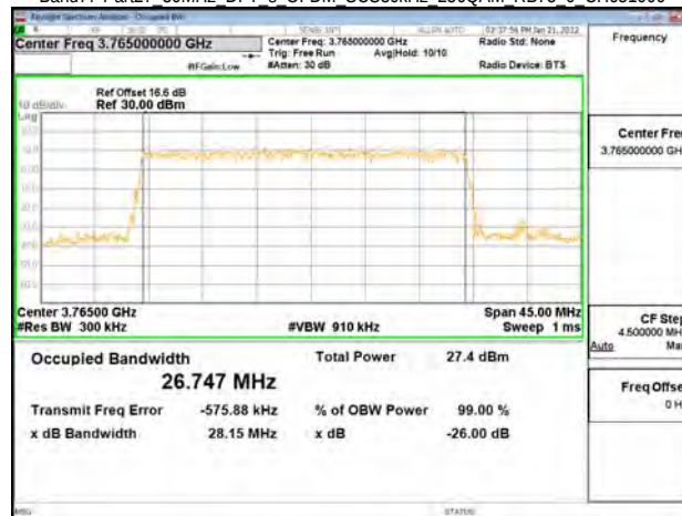
Band77-Part27 30MHz DFT s OFDM SCS30kHz 256QAM RB75 0 CH656000
