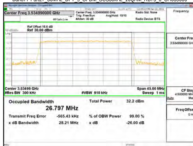
Band77-Part27 30MHz DFT s OFDM SCS30kHz 16QAM RB75 0 CH635666
