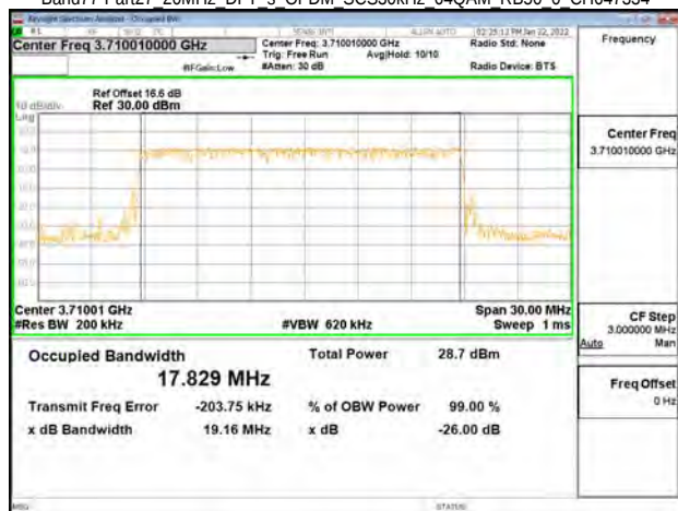
Band77-Part27 20MHz DFT s OFDM SCS30kHz 64QAM RB50 0 CH647334
