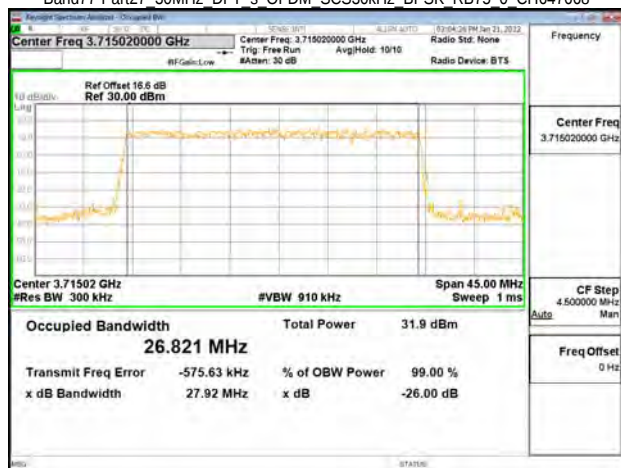
Band77-Part27 30MHz DFT s OFDM SCS30kHz BPSK RB75 0 CH647668
