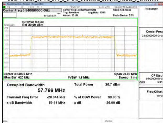
Band77-Part27 60MHz DFT s OFDM SCS30kHz 256QAM RB162 0 CH653332
