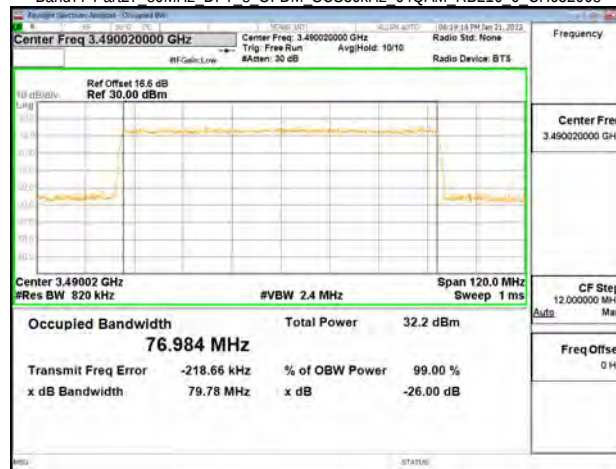
Band77-Part27 80MHz DFT s OFDM SCS30kHz 64QAM RB216 0 CH633334
