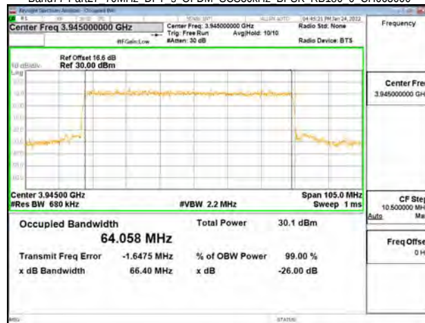
Band77-Part27 70MHz DFT s OFDM SCS30kHz QPSK RB180 0 CH649000
