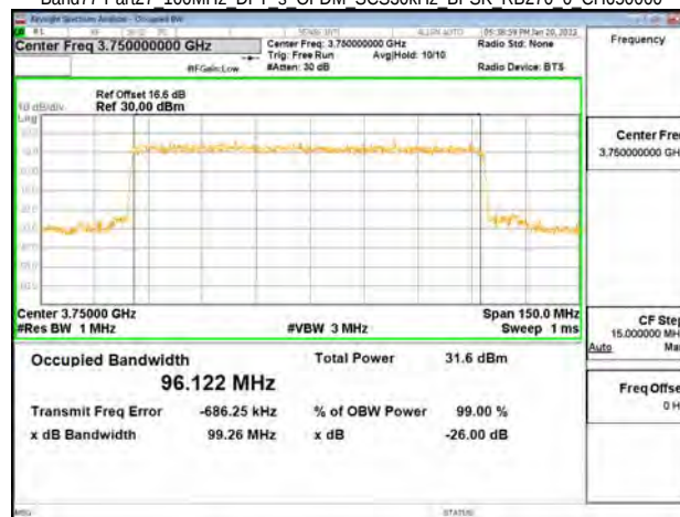
Band77-Part27 100MHz DFT s OFDM SCS30kHz BPSK RB270 0 CH650000
