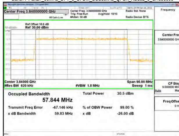
Band77-Part27 60MHz DFT s OFDM SCS30kHz QPSK RB162 0 CH663332
