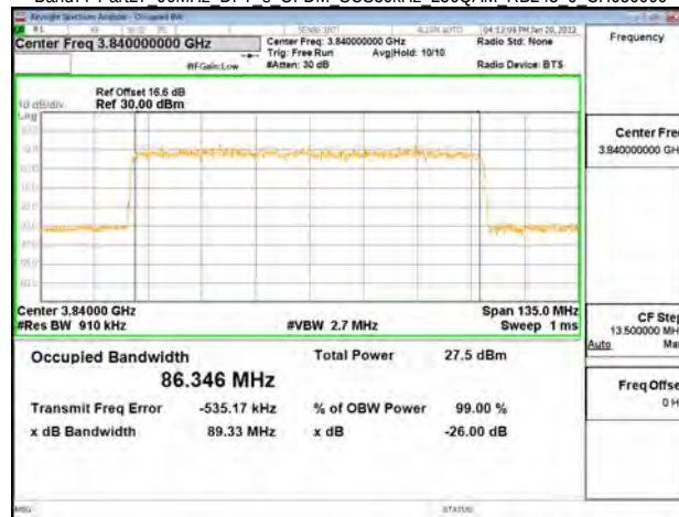
Band77-Part27 90MHz DFT s OFDM SCS30kHz 256QAM RB243 0 CH662332
