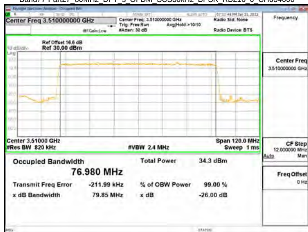
Band77-Part27 80MHz DFT s OFDM SCS30kHz BPSK RB216 0 CH634000
