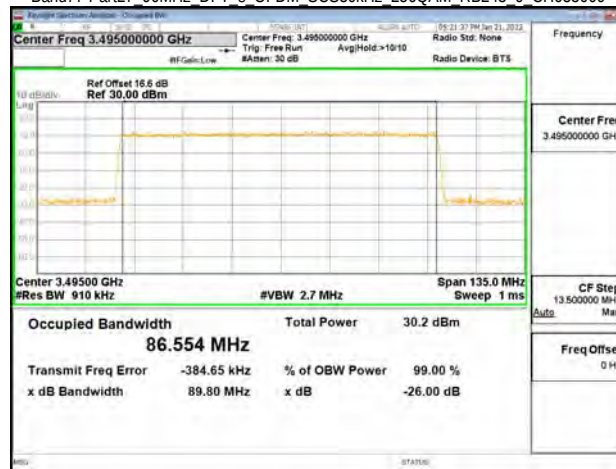
Band77-Part27 90MHz DFT s OFDM SCS30kHz 256QAM RB243 0 CH633334
