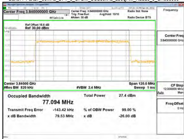
Band77-Part27 80MHz DFT s OFDM SCS30kHz 256QAM RB216 0 CH662666
