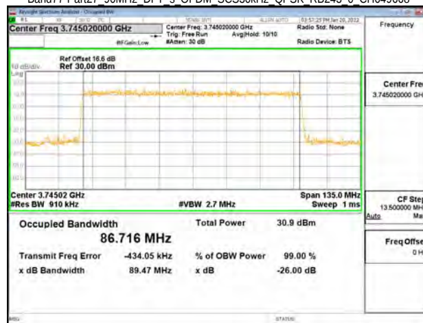
Band77-Part27 90MHz DFT s OFDM SCS30kHz QPSK RB243 0 CH649668
