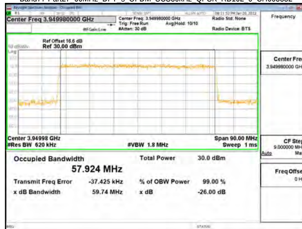
Band77-Part27 60MHz DFT s OFDM SCS30kHz 16QAM RB162 0 CH648668
