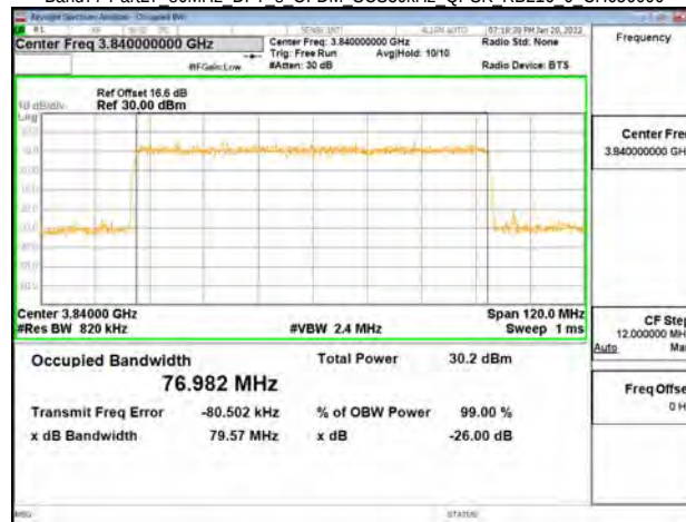
Band77-Part27 80MHz DFT s OFDM SCS30kHz QPSK RB216 0 CH662666
