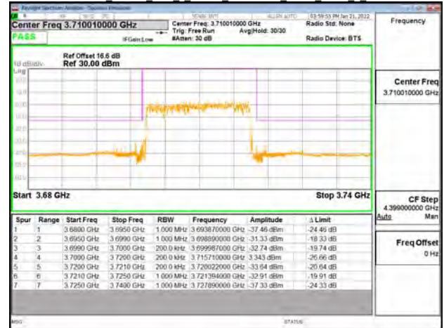
Band77-Part27 20MHz DFT s OFDM SCS30kHz BPSK RB50 0 CH656000
