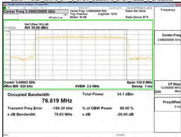
Band77-Part27 80MHz DFT s OFDM SCS30kHz BPSK RB216 0 CH633334
