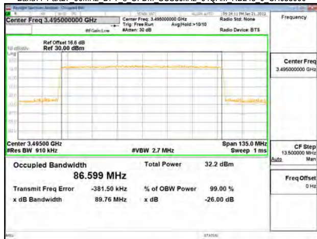
Band77-Part27 90MHz DFT s OFDM SCS30kHz 64QAM RB243 0 CH633334
