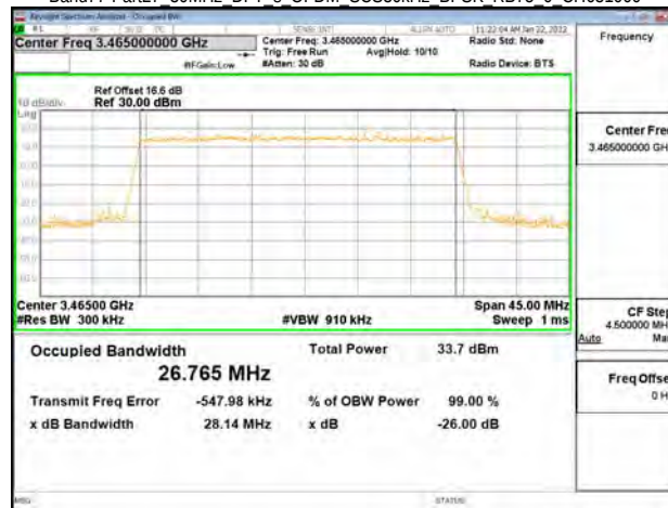
Band77-Part27 30MHz DFT s OFDM SCS30kHz BPSK RB75 0 CH633334
