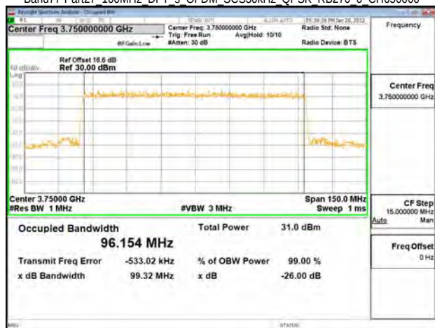
Band77-Part27 100MHz DFT s OFDM SCS30kHz QPSK RB270 0 CH650000
