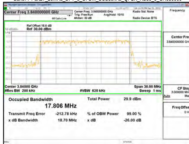
Band77-Part27 20MHz DFT s OFDM SCS30kHz QPSK RB50 0 CH664666
