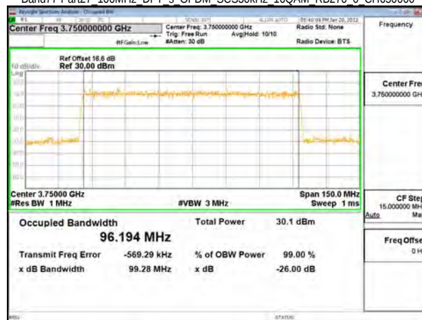
Band77-Part27 100MHz DFT s OFDM SCS30kHz 16QAM RB270 0 CH650000
