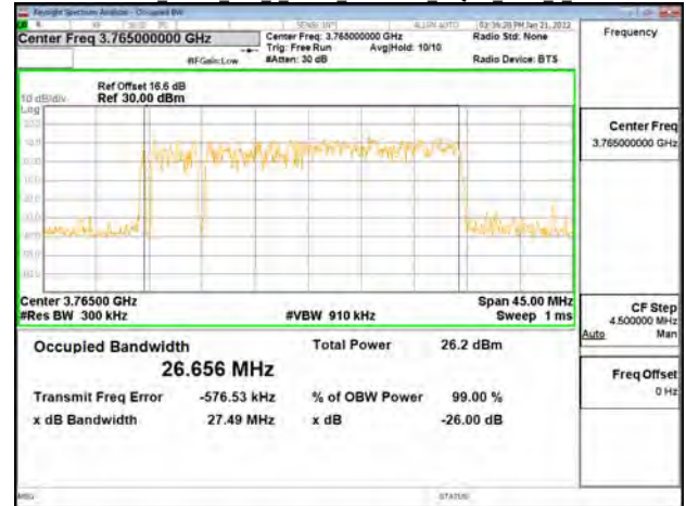
Band77-Part27 30MHz DFT s OFDM SCS30kHz 16QAM RB75 0 CH656000
