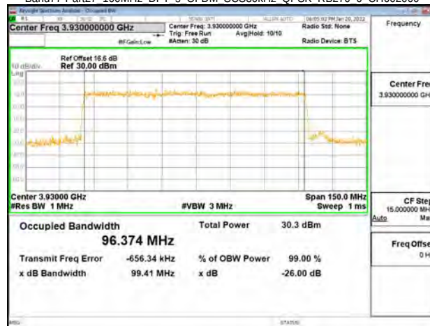
Band77-Part27 100MHz DFT s OFDM SCS30kHz 16QAM RB270 0 CH650000
