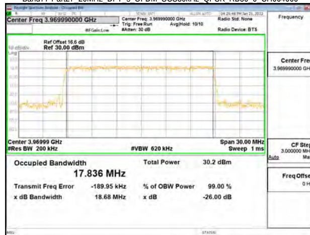
Band77-Part27 20MHz DFT s OFDM SCS30kHz 16QAM RB50 0 CH647334
