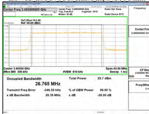
Band77-Part27 30MHz DFT s OFDM SCS30kHz 256QAM RB75 0 CH633334
