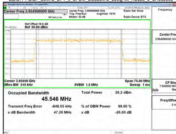
Band77-Part27 60MHz DFT s OFDM SCS30kHz BPSK RB162 0 CH648668
