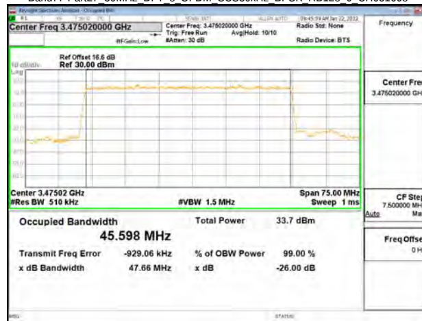
Band77-Part27 50MHz DFT s OFDM SCS30kHz BPSK RB128 0 CH633334
