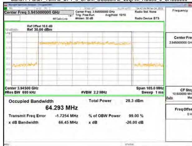
Band77-Part27 70MHz DFT s OFDM SCS30kHz 64QAM RB180 0 CH649000
