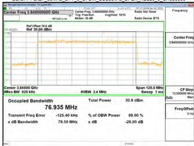
Band77-Part27 80MHz DFT s OFDM SCS30kHz BPSK RB216 0 CH662666
