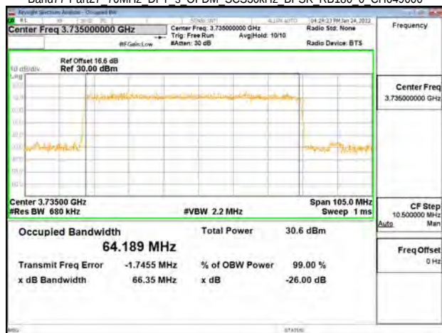
Band77-Part27 70MHz DFT s OFDM SCS30kHz BPSK RB180 0 CH649000
