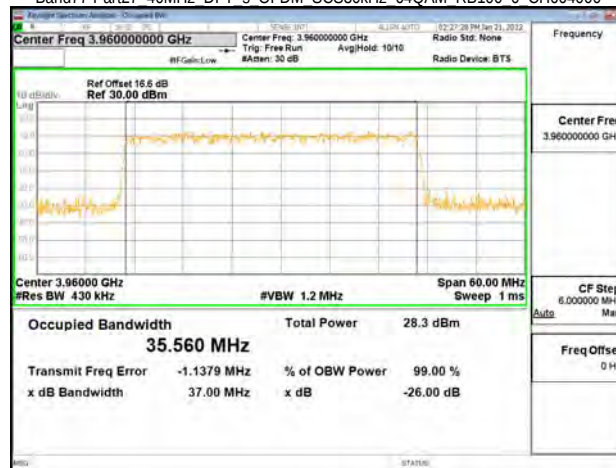
Band77-Part27 40MHz DFT s OFDM SCS30kHz 256QAM RB100 0 CH648000
