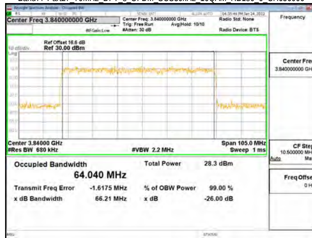
Band77-Part27 70MHz DFT s OFDM SCS30kHz 16QAM RB180 0 CH663000
