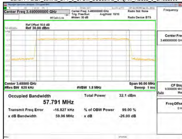
Band77-Part27 60MHz DFT s OFDM SCS30kHz 64QAM RB162 0 CH633334
