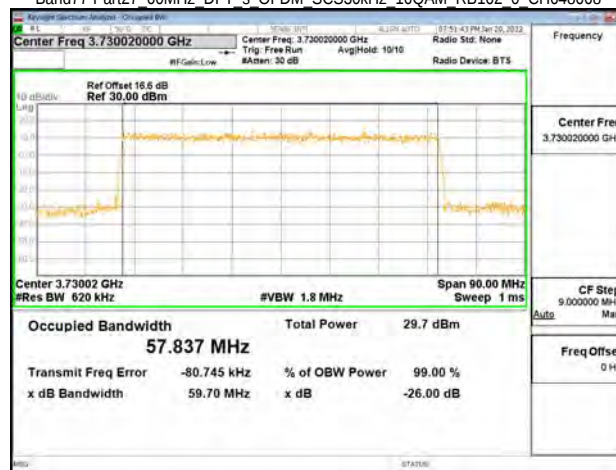
Band77-Part27 60MHz DFT s OFDM SCS30kHz 16QAM RB162 0 CH648668
