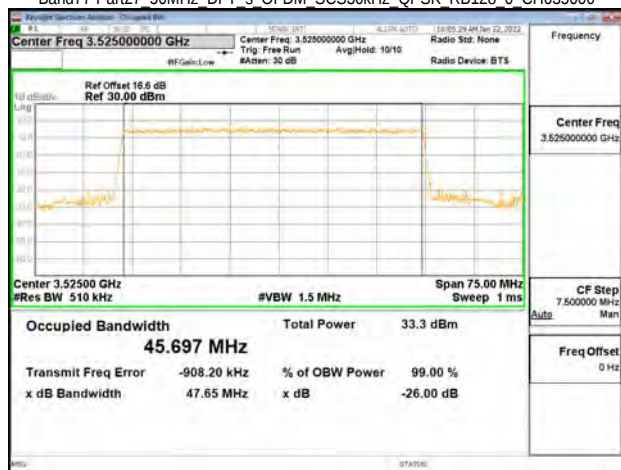
Band77-Part27 50MHz DFT s OFDM SCS30kHz QPSK RB128 0 CH635000
