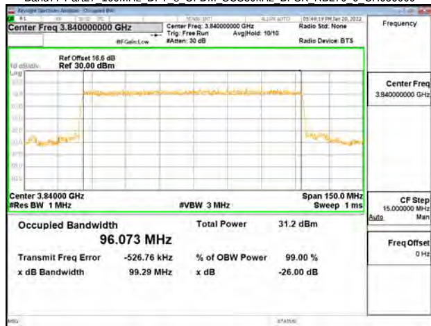
Band77-Part27 100MHz DFT s OFDM SCS30kHz BPSK RB270 0 CH662000
