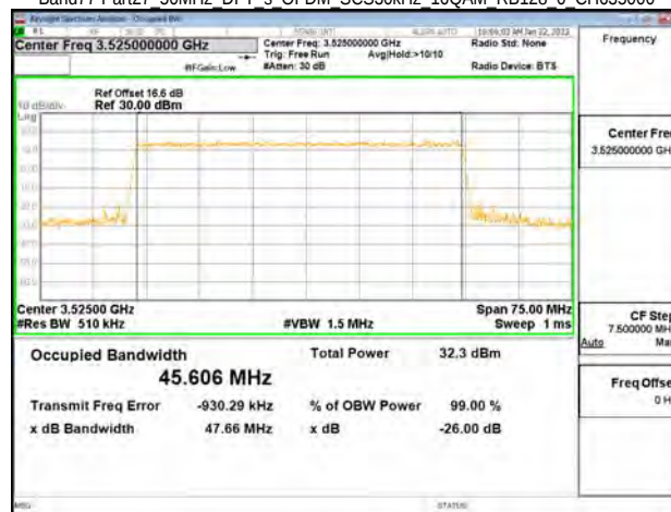
Band77-Part27 50MHz DFT s OFDM SCS30kHz 16QAM BB128 0 CH635000
