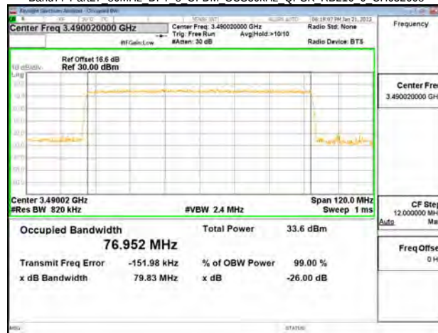
Band77-Part27 80MHz DFT s OFDM SCS30kHz QPSK RB216 0 CH633334
