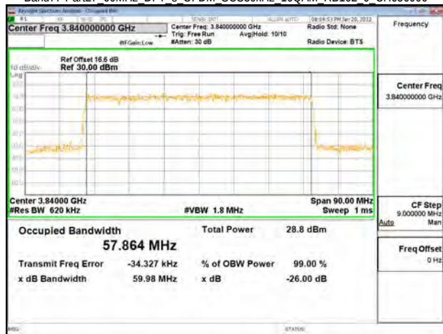
Band77-Part27 60MHz DFT s OFDM SCS30kHz 16QAM RB162 0 CH663332
