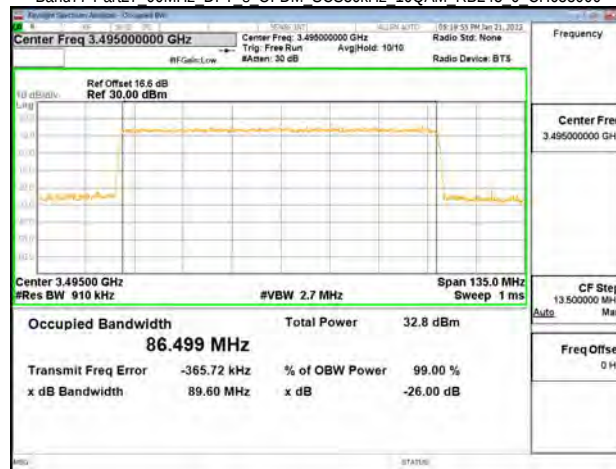
Band77-Part27 90MHz DFT s OFDM SCS30kHz 16QAM RB243 0 CH633334
