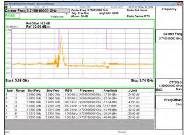
Band77-Part27 20MHz DFT s OFDM SCS30kHz BPSK RB1 0 CH656000
