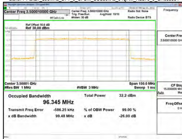
Band77-Part27 100MHz DFT s OFDM SCS30kHz 256QAM RB270 0 CH633334
