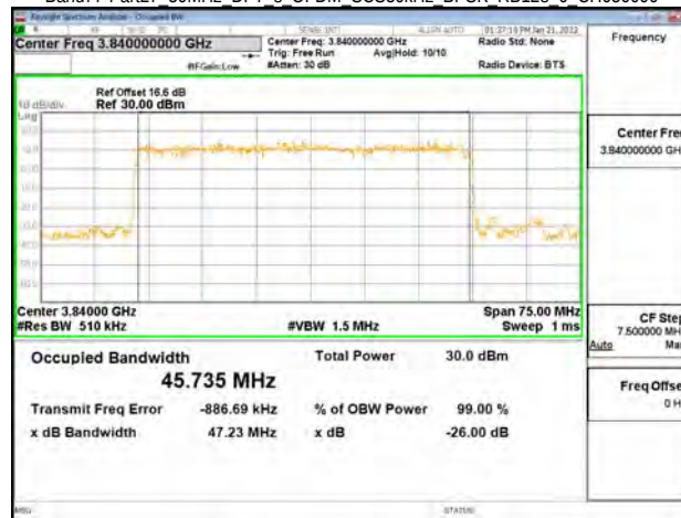
Band77-Part27 50MHz DFT s OFDM SCS30kHz BPSK RB128 0 CH663666
