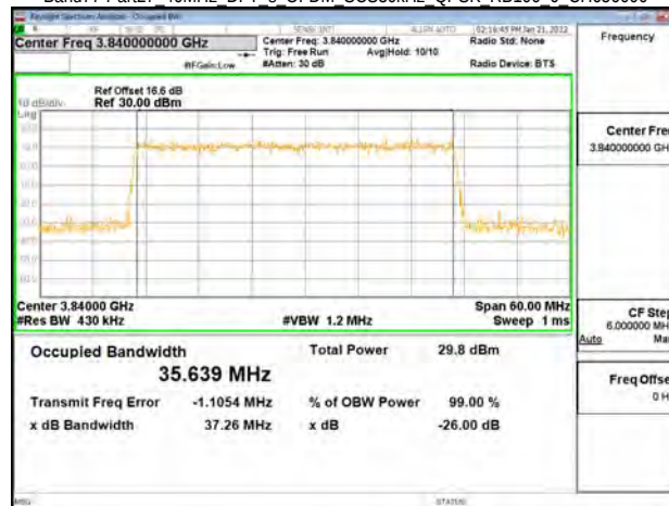
Band77-Part27 40MHz DFT s OFDM SCS30kHz QPSK RB100 0 CH664000
