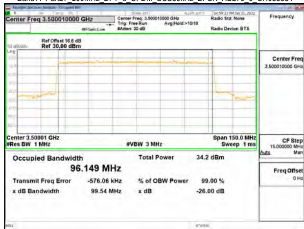
Band77-Part27 100MHz DFT s OFDM SCS30kHz QPSK RB270 0 CH633334
