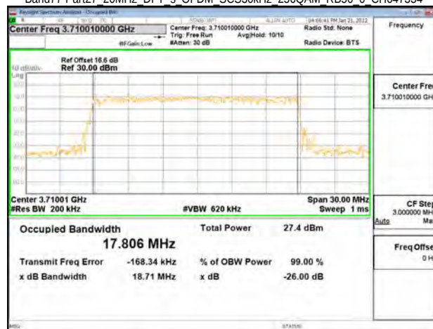
Band77-Part27 20MHz DFT s OFDM SCS30kHz 256QAM RB50 0 CH647334
