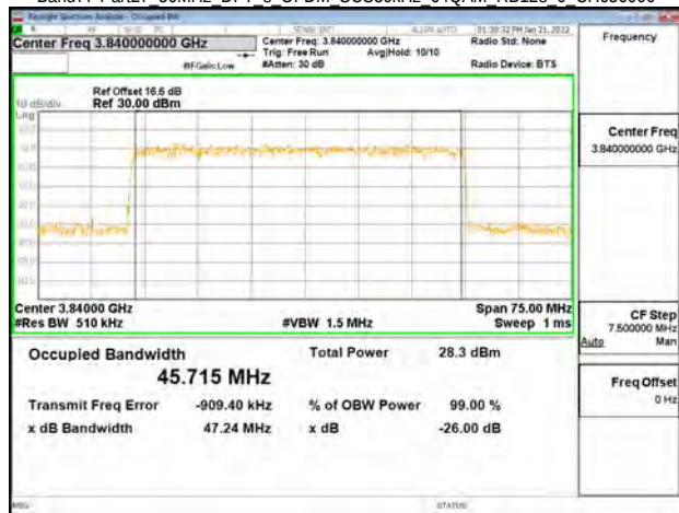
Band77-Part27 50MHz DFT s OFDM SCS30kHz 64QAM RB128 0 CH663666
