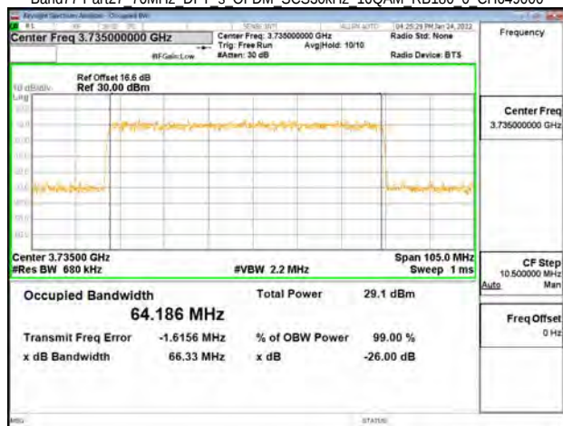
Band77-Part27 70MHz DFT s OFDM SCS30kHz 16QAM RB180 0 CH649000
