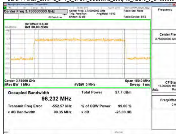
Band77-Part27 100MHz DFT s OFDM SCS30kHz 256QAM RB270 0 CH650000
