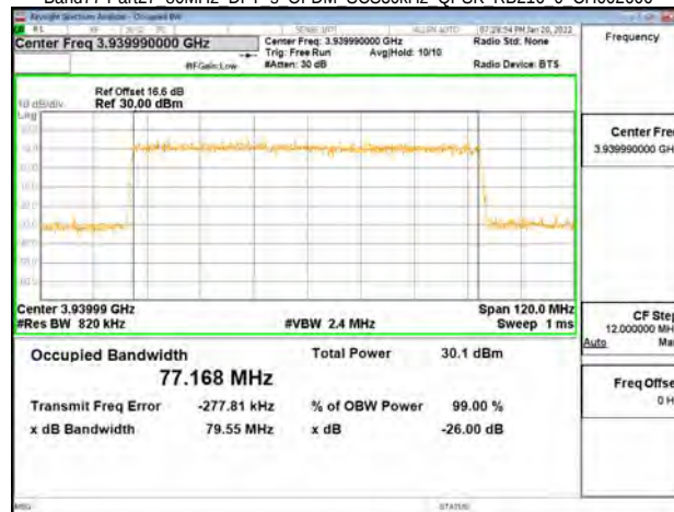
Band77-Part27 80MHz DFT s OFDM SCS30kHz 16QAM RB216 0 CH649334
