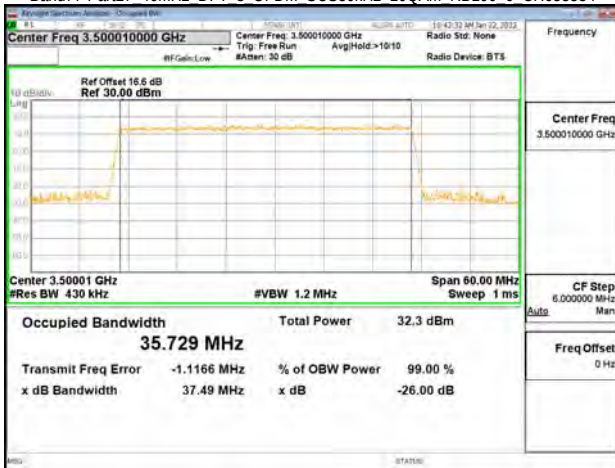
Band77-Part27 40MHz DFT s OFDM SCS30kHz 16QAM RB100 0 CH635332
