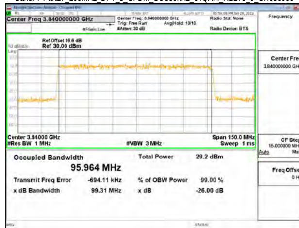
Band77-Part27 100MHz DFT s OFDM SCS30kHz 64QAM RB270 0 CH662000
