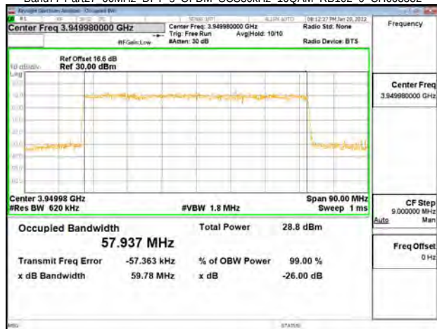
Band77-Part27 60MHz DFT s OFDM SCS30kHz 64QAM RB162 0 CH648668
