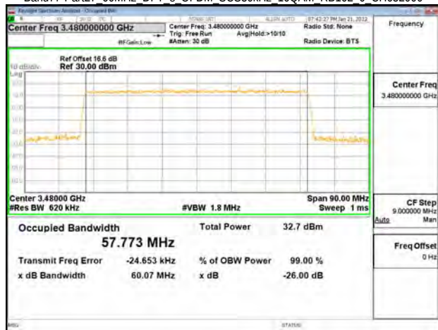
Band77-Part27 60MHz DFT s OFDM SCS30kHz 16QAM RB162 0 CH633334
