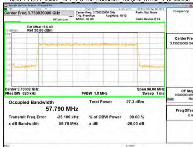
Band77-Part27 60MHz DFT s OFDM SCS30kHz 256QAM RB162 0 CH648668
