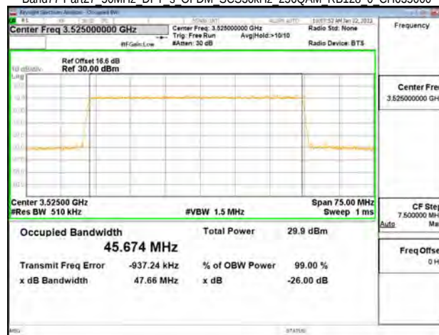
Band77-Part27 50MHz DFT s OFDM SCS30kHz 256QAM RB128 0 CH635000
