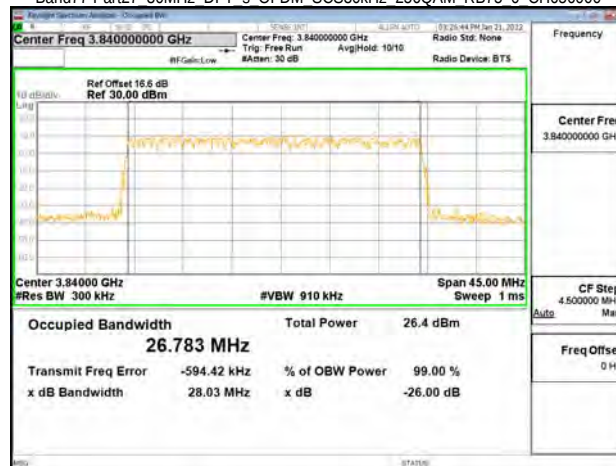
Band77-Part27 40MHz DFT s OFDM SCS30kHz BPSK RB100 0 CH648000
