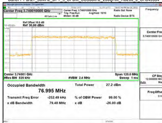
Band77-Part27 80MHz DFT s OFDM SCS30kHz 256QAM RB216 0 CH649334
