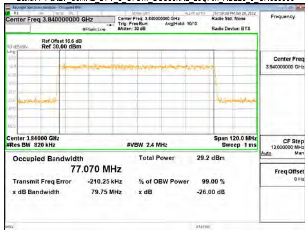
Band77-Part27 80MHz DFT s OFDM SCS30kHz 16QAM RB216 0 CH662666
