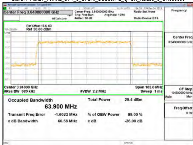
Band77-Part27 70MHz DFT s OFDM SCS30kHz QPSK RB180 0 CH663000
