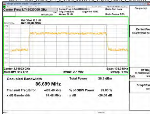
Band77-Part27 90MHz DFT s OFDM SCS30kHz 64QAM RB243 0 CH649668
