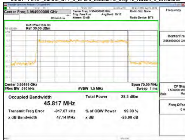
Band77-Part27 50MHz DFT s OFDM SCS30kHz 64QAM RB128 0 CH648334
