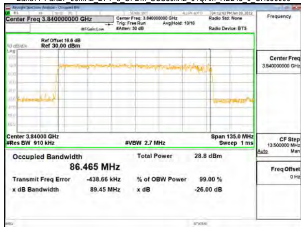
Band77-Part27 90MHz DFT s OFDM SCS30kHz 64QAM RB243 0 CH662332
