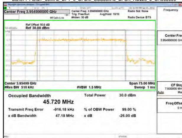
Band77-Part27 50MHz DFT s OFDM SCS30kHz QPSK RB128 0 CH648334
