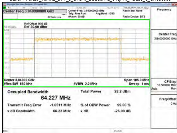
Band77-Part27 70MHz DFT s OFDM SCS30kHz 64QAM RB180 0 CH663000
