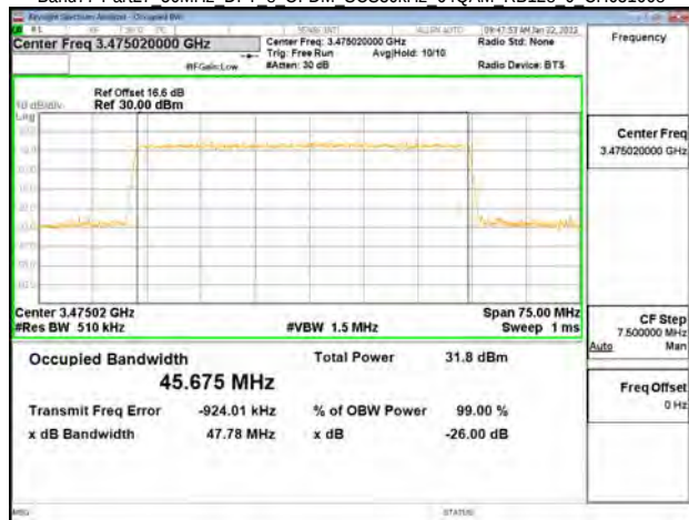
Band77-Part27 50MHz DFT s OFDM SCS30kHz 64QAM RB128 0 CH633334
