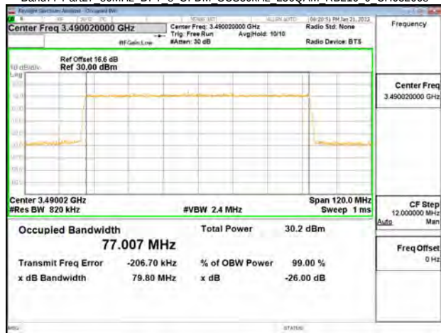
Band77-Part27 80MHz DFT s OFDM SCS30kHz 256QAM RB216 0 CH633334
