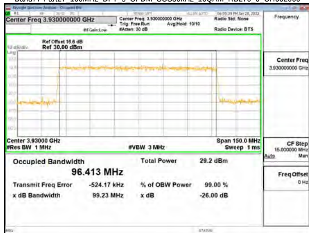
Band77-Part27 100MHz DFT s OFDM SCS30kHz 64QAM RB270 0 CH650000
