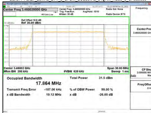
Band77-Part27 20MHz DFT s OFDM SCS30kHz 64QAM RB50 0 CH633334
