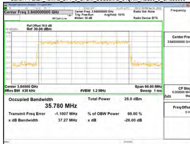
Band77-Part27 40MHz DFT s OFDM SCS30kHz 64QAM RB100 0 CH664000
