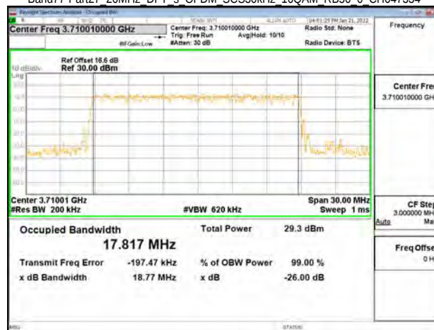
Band77-Part27 20MHz DFT s OFDM SCS30kHz 16QAM RB50 0 CH647334
