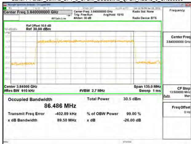
Band77-Part27 90MHz DFT s OFDM SCS30kHz QPSK RB243 0 CH662332
