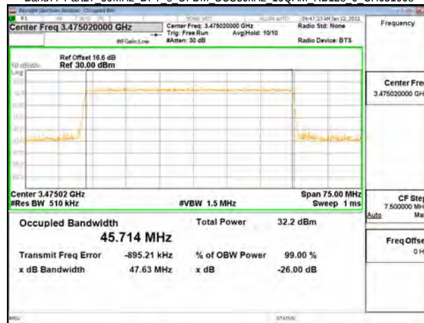
Band77-Part27 50MHz DFT s OFDM SCS30kHz 16QAM RB128 0 CH6333334
