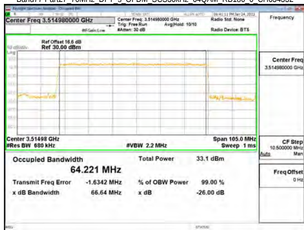
Band77-Part27 70MHz DFT s OFDM SCS30kHz 64QAM RB180 0 CH634332
