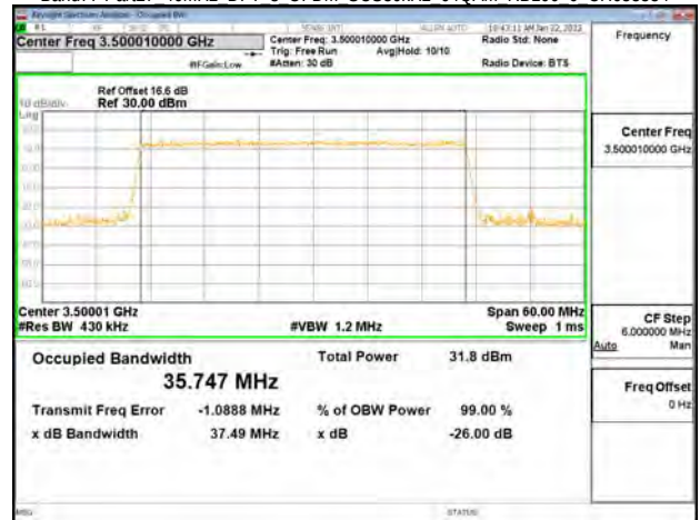
Band77-Part27 40MHz DFT s OFDM SCS30kHz 64QAM RB100 0 CH635332
