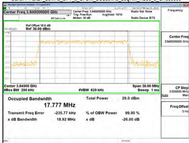
Band77-Part27 20MHz DFT s OFDM SCS30kHz 16QAM RB50 0 CH664666
