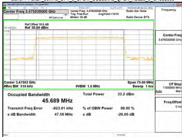
Band77-Part27 50MHz DFT s OFDM SCS30kHz OPSK RB128 0 CH6333334
