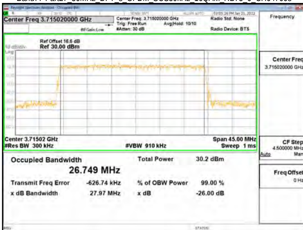
Band77-Part27 30MHz DFT s OFDM SCS30kHz 16QAM RB75 0 CH647668
