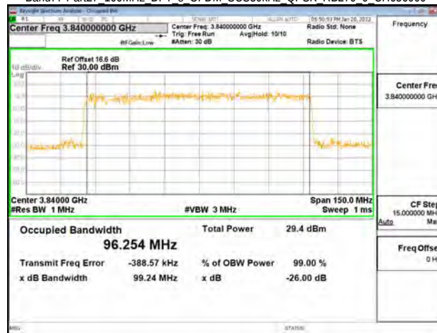
Band77-Part27 100MHz DFT s OFDM SCS30kHz QPSK RB270 0 CH662000
