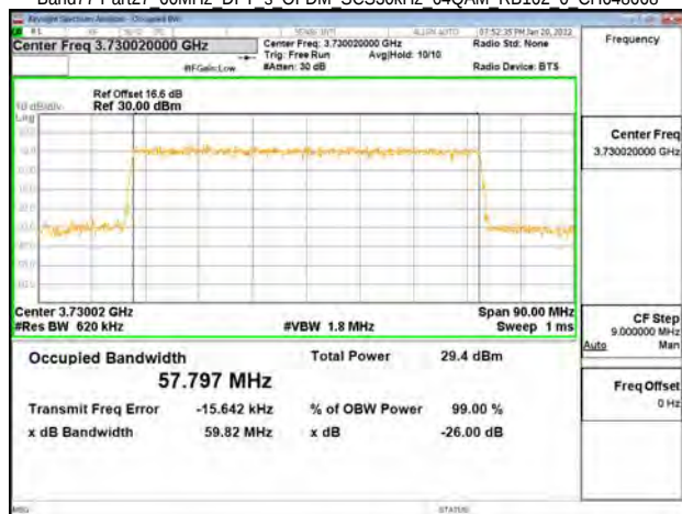
Band77-Part27 60MHz DFT s OFDM SCS30kHz 64QAM RB162 0 CH648668
