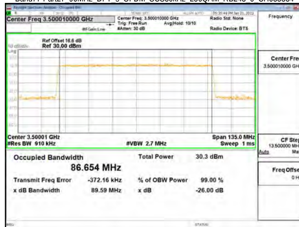
Band77-Part27 90MHz DFT s OFDM SCS30kHz 256QAM RB243 0 CH633666
