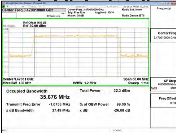
Band77-Part27 40MHz DFT s OFDM SCS30kHz 16QAM RB100 0 CH633334
