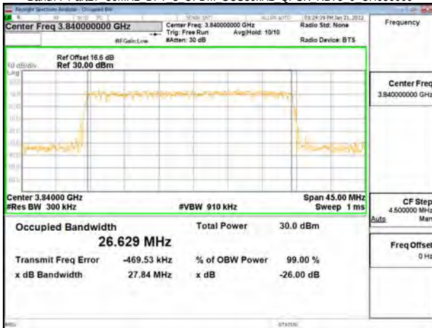
Band77-Part27 30MHz DFT s OFDM SCS30kHz 16QAM RB75 0 CH647668
