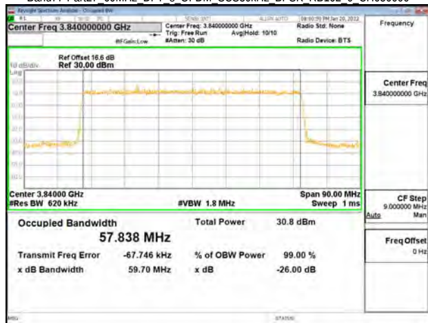
Band77-Part27 60MHz DFT s OFDM SCS30kHz BPSK RB162 0 CH663332
