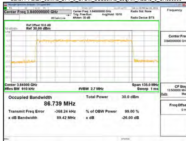
Band77-Part27 90MHz DFT s OFDM SCS30kHz 16QAM RB243 0 CH662332
