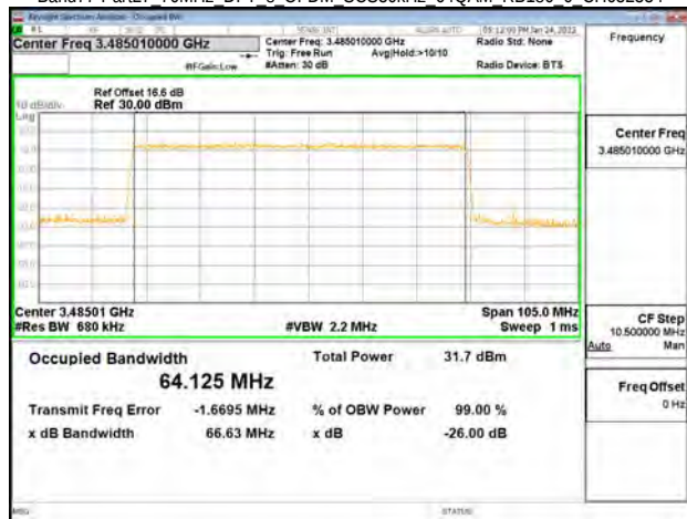
Band77-Part27 70MHz DFT s OFDM SCS30kHz 64QAM RB180 0 CH633334
