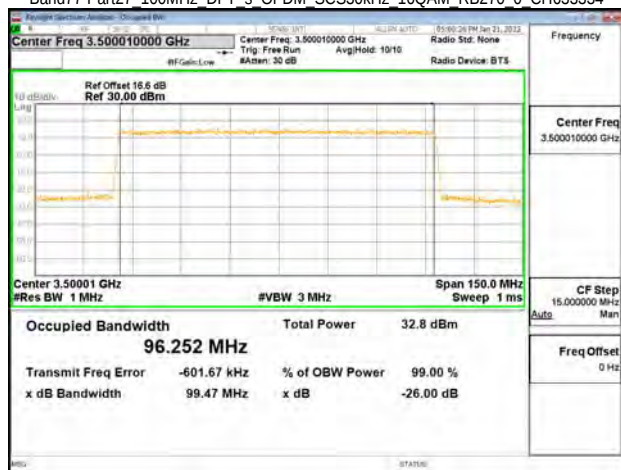
Band77-Part27 100MHz DFT s OFDM SCS30kHz 16QAM RB270 0 CH633334
