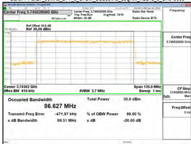
Band77-Part27 90MHz DFT s OFDM SCS30kHz 16QAM RB243 0 CH649668
