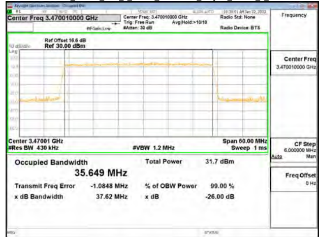
Band77-Part27 40MHz DFT s OFDM SCS30kHz 64QAM RB100 0 CH633334
