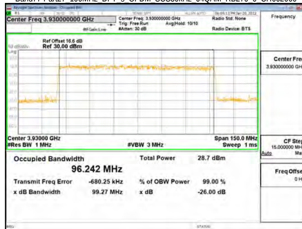
Band77-Part27 100MHz DFT s OFDM SCS30kHz 256QAM RB270 0 CH650000
