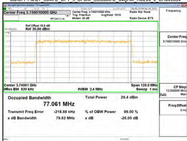
Band77-Part27 80MHz DFT s OFDM SCS30kHz 64QAM RB216 0 CH649334
