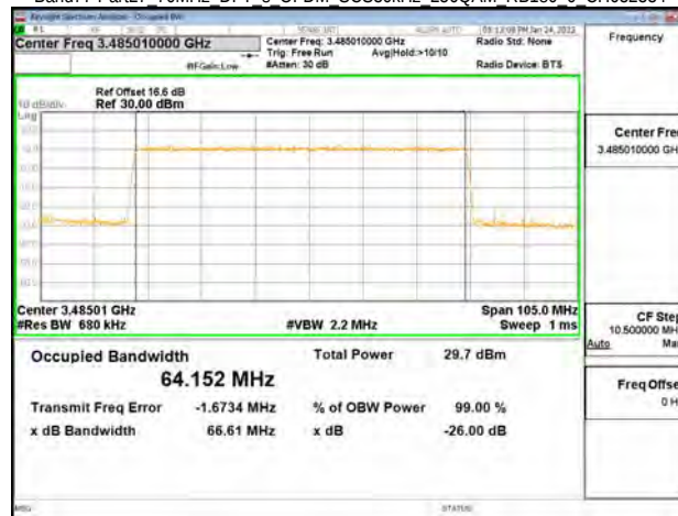
Band77-Part27 70MHz DFT s OFDM SCS30kHz 256QAM RB180 0 CH633334
