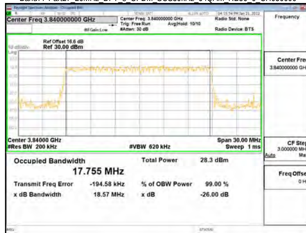
Band77-Part27 20MHz DFT s OFDM SCS30kHz 64QAM RB50 0 CH664666
