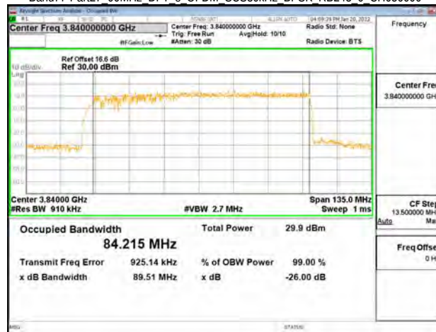
Band77-Part27 90MHz DFT s OFDM SCS30kHz BPSK RB243 0 CH662332
