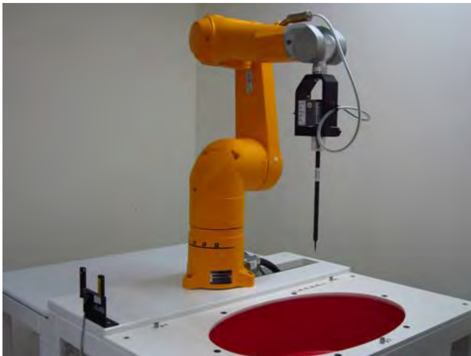
Fig.1 Photograph of the SAR measurement system
