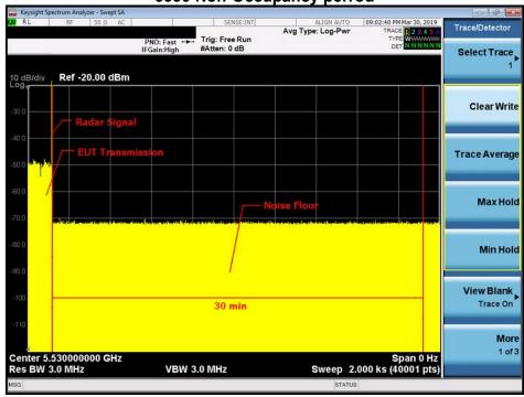
TX AC (VHT160) Mode 5570 Non-Occupancy perrod
